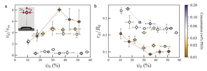
Fig. 8 Non-dimensionalized top jet drop (a) velocity and (b) radius as a function of compound layer volume fraction with PEO concentrations of 0.01–0.1 wt% under which jet drops form.
