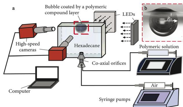
**Fig. 1** (a) Experimental setup for high-speed imaging for the jetting dynamics of bubbles with a viscoelastic compound interface. (b) Zoomed-in image of a typical compound bubble coated by a polymeric layer.  $R_0$  is the compound bubble radius.
