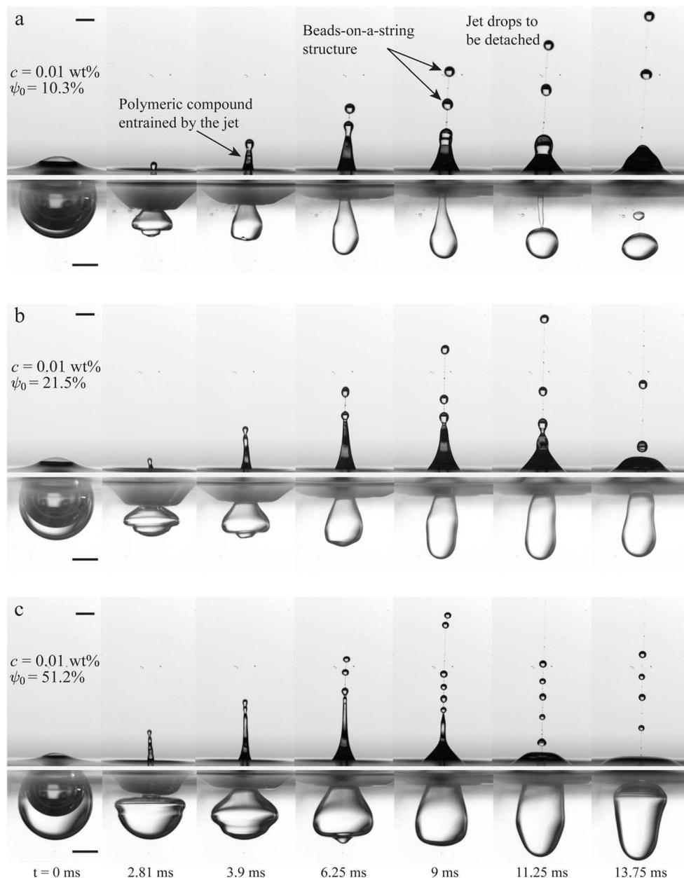
Fig. 5 Side view of a bursting bubble coated by a compound layer at a PEO concentration of 0.01 wt% for (a)  $\psi_0 = 10.3\%$ , (b)  $\psi_0 = 21.5\%$ , and (c)  $\psi_0 = 51.2\%$ . During the rising of the jet, the end-pinching instability causes it to break up into drops and form a beads-on-a-string structure. All scale bars represent 1 mm. See also ESI Videos 3 and 4† corresponding to (a).
