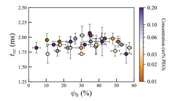
Fig. 4 Cavity collapse time  $t_{\rm cc}$  as a function of  $\psi_0$  for bursting bubbles coated by PEO solutions with concentrations of 0.01–0.2 wt%. The collapse time across all cases remains nearly constant, with a value of 1.88  $\pm$  0.11 ms.
