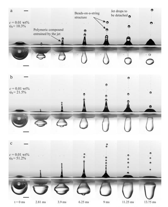
Fig. 5 Side view of a bursting bubble coated by a compound layer at a PEO concentration of 0.01 wt% for (a)  $\psi_0=10.3\%$ , (b)  $\psi_0=21.5\%$ , and (c)  $\psi_0=51.2\%$ . During the rising of the jet, the end-pinching instability causes it to break up into drops and form a beads-on-a-string structure. All scale bars represent 1 mm. See also ESI Videos 3 and 4† corresponding to (a).
