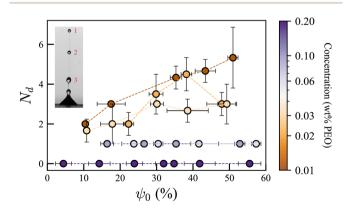
Fig. 9 Number of jet drops,  $N_{\rm d}$ , as a function of compound layer volume fractions with different PEO concentrations of 0.01–0.2 wt%. The inset illustrates an example featuring three jet drops.
