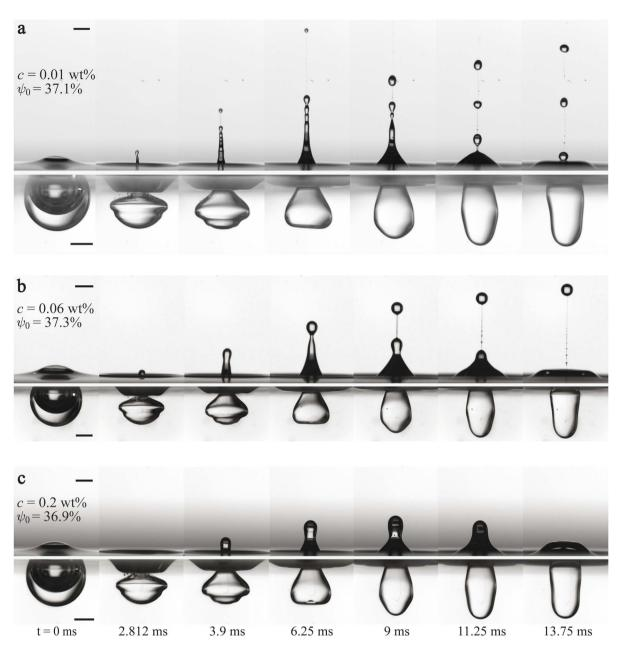
Fig. 6 Side view of a bursting bubble coated by a compound layer at a PEO concentration of (a) c=0.01 wt%, (b) c=0.06 wt%, and (c) c=0.2 wt% for  $\psi_0\approx 37\%$ . As c increases while maintaining a nearly constant  $\psi_0$ , we observe a transition in compound bubble bursting behavior from generating jet drops to producing no jet drops. All scale bar represents 1 mm.
