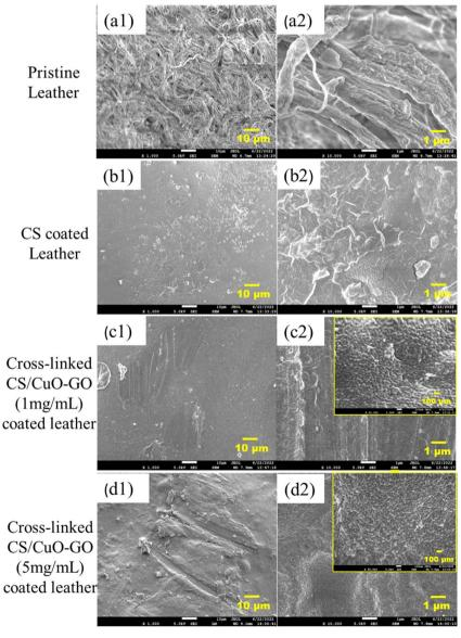
Fig. 4 FE-SEM images of pristine leather (a1 and a2), chitosan-coated leather (b1 and b2), CS/CuO-GO (1 mg mL $^{-1}$ ) coated leather (c1 and c2), and CS/CuO-GO (5 mg mL $^{-1}$ ) coated leather (d1 and d2) samples at different magnifications (1000× and 10000×). Insets show magnified images (50000×), indicating the presence of CuO-GO nanostructure on the leather surface.
