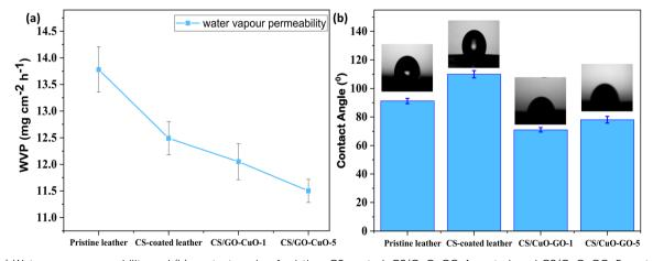
Fig. 11 (a) Water vapor permeability and (b) contact angle of pristine, CS coated, CS/CuO-GO-1 coated, and CS/CuO-GO-5 coated leather samples.
