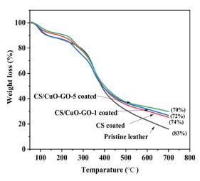
Fig. 6 TGA thermogram of pristine leather, CS-coated leather, CS/CuO-GO (1 mg  $\rm mL^{-1}$ ), and CS/CuO-GO (5 mg  $\rm mL^{-1}$ ) nanocomposite-coated leather.
