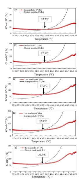
Fig. 7 Dependence of G' and G'' on the temperature increase for various MC/HA-Me conjugates hydrogels with the content of MC from 5.0 wt% to 7.0 wt% increase at constant of 4.5%HA-Me/1.0% NaCl: (a) 5.0 wt%-MC, (b) 5.5 wt%-MC (c) 6.0 wt%-MC (d) 6.5 wt%-MC (e) 7.0 wt%-MC.
