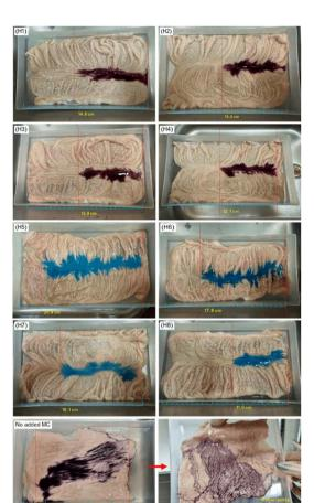
Fig. 8 The gelation time and flow distance of various hydrogel formulations were evaluated using an ultrasonic oscillator in an in vitro simulation through porcine intestine at a constant temperature and frequency (37 °C and 20 Hz). H1-H4 hydrogel formulations: 6.5% MC mixed with 4.0%, 4.5%, 5.0% and 6.0% HAMe, respectively; H5-H8 hydrogel formulations: 4.5% HAMe mixed with 5.0%, 5.5%, 6.0% and 7.0% MC, respectively; no added MC: 4.5% HAMe.
