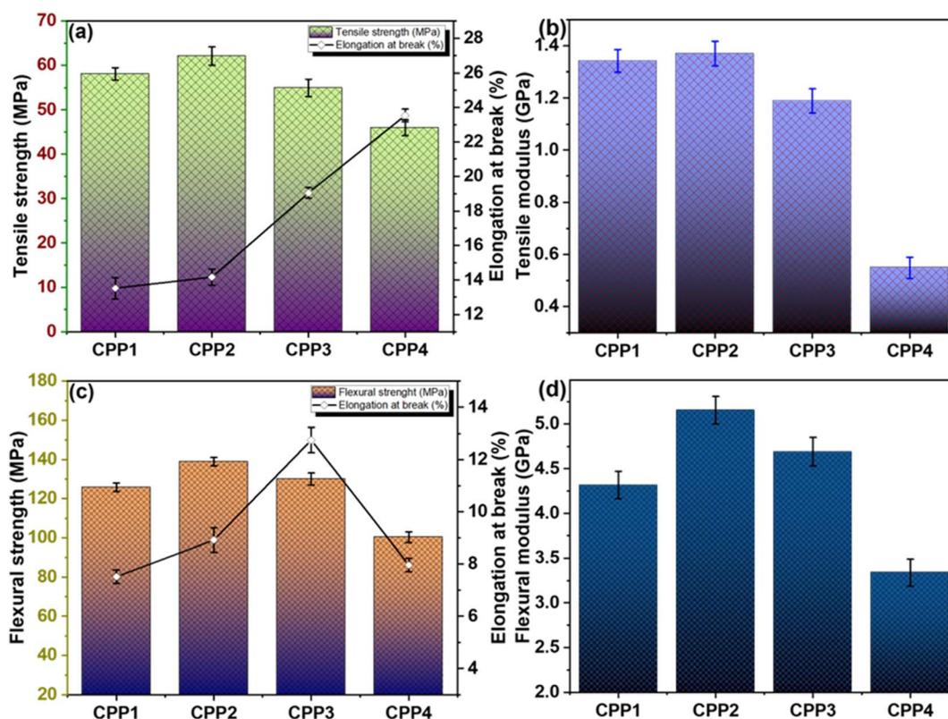
Fig. 2 Mechanical properties of developed cotton-reinforced PP composites; (a) tensile strength and breaking extension, (b) tensile modulus, (c) flexural strength and breaking extension and (d) flexural modulus.
