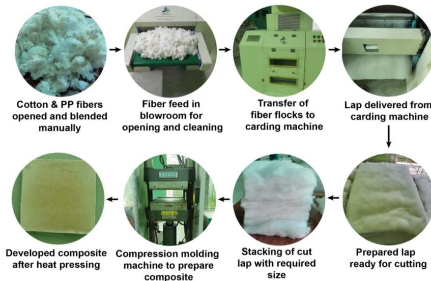
**Fig. 1** Schematic diagram of developing cotton–PP composite through uniform blending of reinforced cotton and PP fibers.
