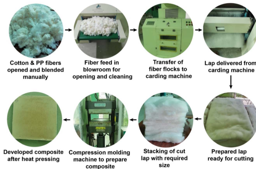
Fig. 1 Schematic diagram of developing cotton–PP composite through uniform blending of reinforced cotton and PP fibers.
