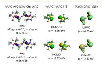
Fig. 4 The shape of the deformation densities  $\Delta \rho_{(1)-(2)}$  that correspond to  $\Delta E_{orb(1)-(2)}$ , and the associated MOs of cAAC-Al(Cl)<sub>2</sub>OAl(Cl)<sub>2</sub>cAAC (1) and the fragments orbitals of [(cAAC)(cAAC)] and [Al(Cl)2-OAI(CI)<sub>2</sub>] in the singlet state (S) at the BP86-D3(BJ)/TZ2P level. Isosurface values are 0.003 au for  $\Delta \rho_{(1)-(2)}$ . The eigenvalues  $|\nu_n|$  give the size of the charge migration in e.
