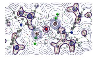
Fig. 7 Contour plot of Laplacian distribution  $[\nabla^2 \rho(r)]$  in the Al3–O4–Al30 plane of  $(cAAC^{Dipp})Al(Cl_2)-O-Al(Cl_2)(cAAC^{Dipp})$  (1'). Solid blue lines indicate the areas of charge concentration  $(\nabla^2 \rho(r) < 0)$  while dotted purple lines denotes charge depletion  $(\nabla^2 \rho(r) > 0)$ . Solid lines connecting atomic nuclei (black) are the bond paths and green spheres on bond path indicates the BCP.
