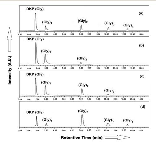
Fig. 7 HPLC chromatogram showing the products formed on the surface of (a) MnHCCo, (b) FeHCCo, (c) NiHCCo, (d) ZnHCCo when glycine was heated at 90 °C after four weeks. Retention times of analyzed products (min): Cyc (Gly)<sub>2</sub> (1.94), Gly (3.04), (Gly)<sub>2</sub> (7.12), (Gly)<sub>3</sub> (10.17), (Gly)<sub>4</sub> (12.35).
