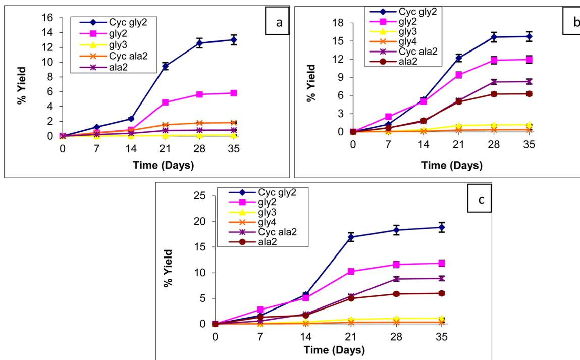
Fig. 6 Oligomerization of amino acid on ZnHCCo complexes at [a] 60 °C, [b] 90 °C, [c] 120 °C.
