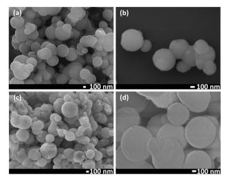
Fig. 2 SEM images of (a) nMCM-48, (b) GLP/nMCM-48, (c) TPA/GLP/MCM-48 and (d) MTF/TPA/GLP/nMCM-48.
