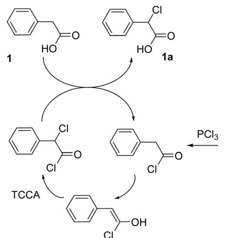
**Scheme 1** Proposed reaction mechanism of  $\alpha$ -chlorination of phenylacetic acid with TCCA in the presence of  $\text{PCl}_3$  under solvent-free conditions.
