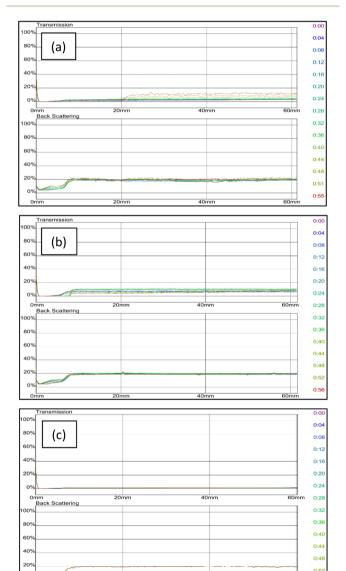
Fig. 13 Transmission and backscattering profiles of grafted bentonite modified with zeolites with (a) Span 80 (b) Tween 80, and (c) combined Span 80 and Tween 80.
