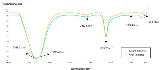
**Fig. 3** FTIR spectra of grafted bentonite before and after immersing in high salinity carbonates.
