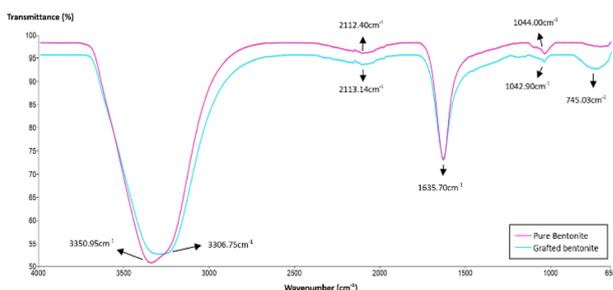
**Fig. 1** FTIR spectra of pure bentonite and grafted bentonite.
