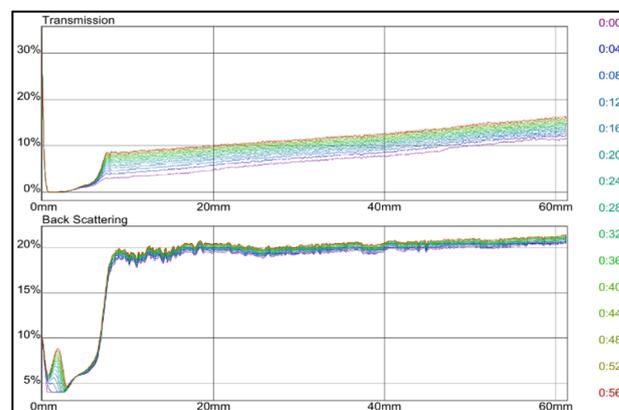
Fig. 7 Transmission and backscattering profiles of pure bentonite.
