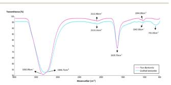
Fig. 1 FTIR spectra of pure bentonite and grafted bentonite.
