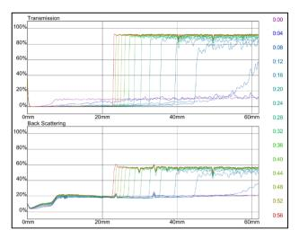
Fig. 10 Transmission and backscattering profiles of bentonite polymerized with AM 58%: 42% AMPS.
