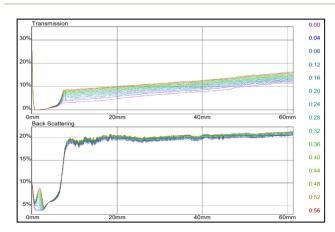
Fig. 7 Transmission and backscattering profiles of pure bentonite.
