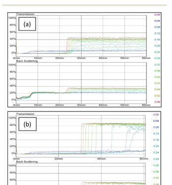
Fig. 12 Transmission and backscattering profiles of grafted bentonite modified with (a) zeolites and (b) zeolites with SDS.
