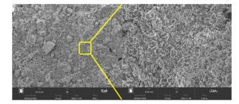
Fig. 6 SEM images of the grafted bentonite in carbonate rocks.
