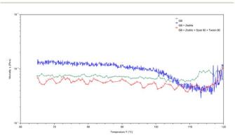
Fig. 15 Effect of temperature on viscosity of GB and modified GB.
