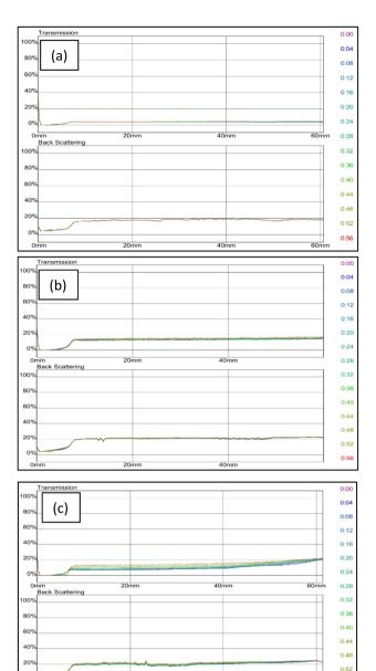
Fig. 11 Transmission and backscattering profiles at (a) 0 wt%, (b) 2.5 wt% and (c) 3.5 wt% NaCl of grafted bentonite.
