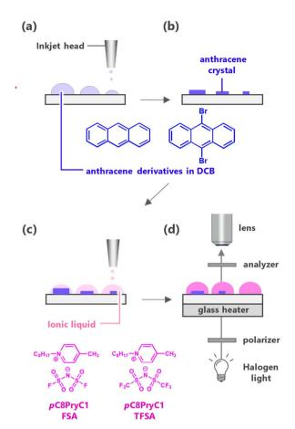
Fig. 1 Schematic for preparing a dot array, consisting of anthracene in an ionic liquid, by inkjet printing for simultaneous screening and construction of a phase diagram. (a) Printing of anthracene in DCB solution, (b) formation of anthracene crystals after air drying, (c) printing of pC8PryC1 derivatives on anthracene derivative crystals, and (d) microscopy observation of anthracene crystal dissolution at the heating stage.
