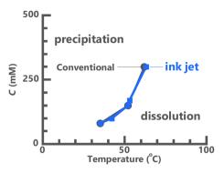
Fig. 5 Phase diagrams of anthracene in pC8PryC1 FSA by applying the inkjet (blue square) and conventional (gray circle) techniques, at pC8PryC1 FSA volumes of 25–100 nL and 0.5–1.0 mL, respectively, at heating rates of 0.20 °C min<sup>-1</sup> and 0.017 °C min<sup>-1</sup>, respectively. Anthracene solutions and pC8PryC1 FSA were ejected under the optimized conditions depicted in Fig. 3.
