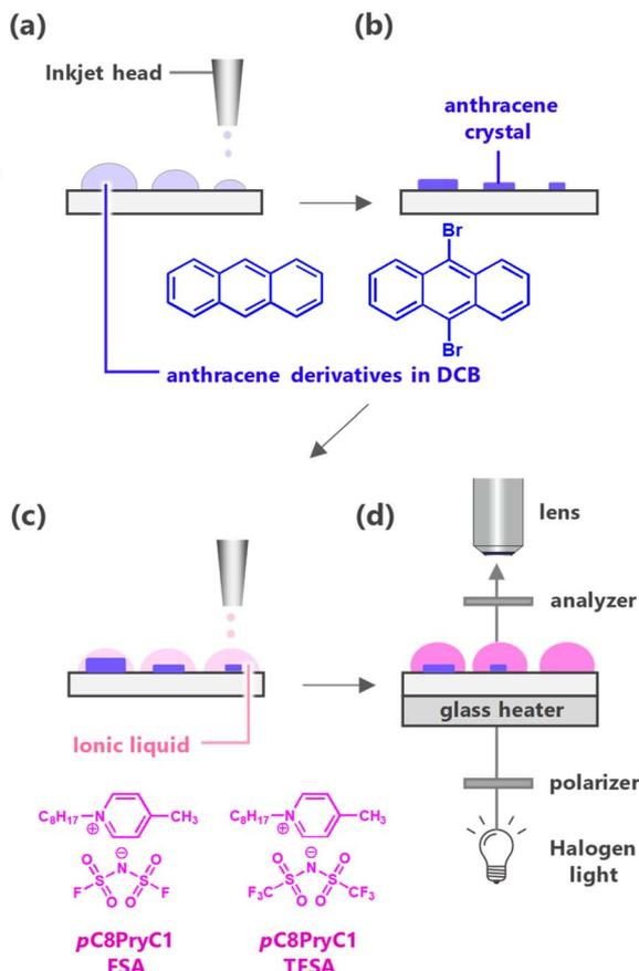
Fig. 1 Schematic for preparing a dot array, consisting of anthracene in an ionic liquid, by inkjet printing for simultaneous screening and construction of a phase diagram. (a) Printing of anthracene in DCB solution, (b) formation of anthracene crystals after air drying, (c) printing of *p*C8PryC1 derivatives on anthracene derivative crystals, and (d) microscopy observation of anthracene crystal dissolution at the heating stage.
