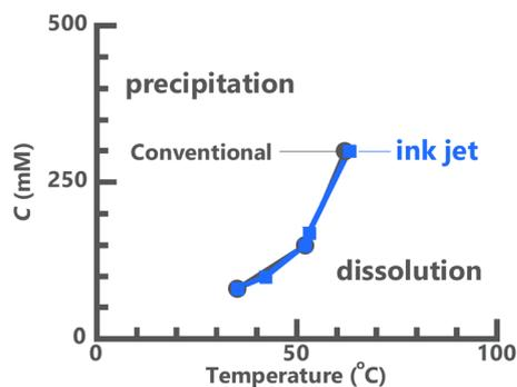
Fig. 5 Phase diagrams of anthracene in *pC8PryC1* FSA by applying the inkjet (blue square) and conventional (gray circle) techniques, at *pC8PryC1* FSA volumes of 25–100 nL and 0.5–1.0 mL, respectively, at heating rates of 0.20 °C min<sup>-1</sup> and 0.017 °C min<sup>-1</sup>, respectively. Anthracene solutions and *pC8PryC1* FSA were ejected under the optimized conditions depicted in Fig. 3.
