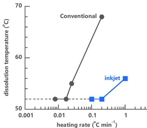
**Fig. 4** Dissolution temperatures of anthracene in *p*C8PryC1 FSA at 150 mM plotted against heating rates. The volumes of *p*C8PryC1 FSA were 0.5 mL and 34 nL for the conventional (gray circle) and inkjet (blue square) techniques, respectively. The dissolution temperature was the temperature at which the crystals were completely dissolved during observation with the unaided eye using the conventional technique or with a microscope using the inkjet technique.
