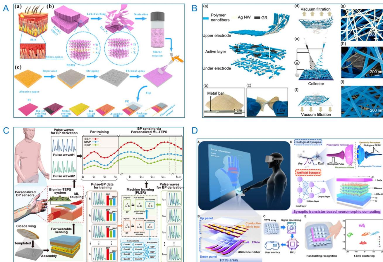
**Fig. 2** (A) Flexible pressure sensor based on MXene nanomaterials.<sup>27</sup> (B) Fabric sensor based on Ag nanofibers.<sup>28</sup> (C) Pulse sensor for continuous blood pressure monitoring.<sup>29</sup> (D) Machine learning-assisted triboelectric-capacitive coupled tactile sensor.<sup>22</sup>
