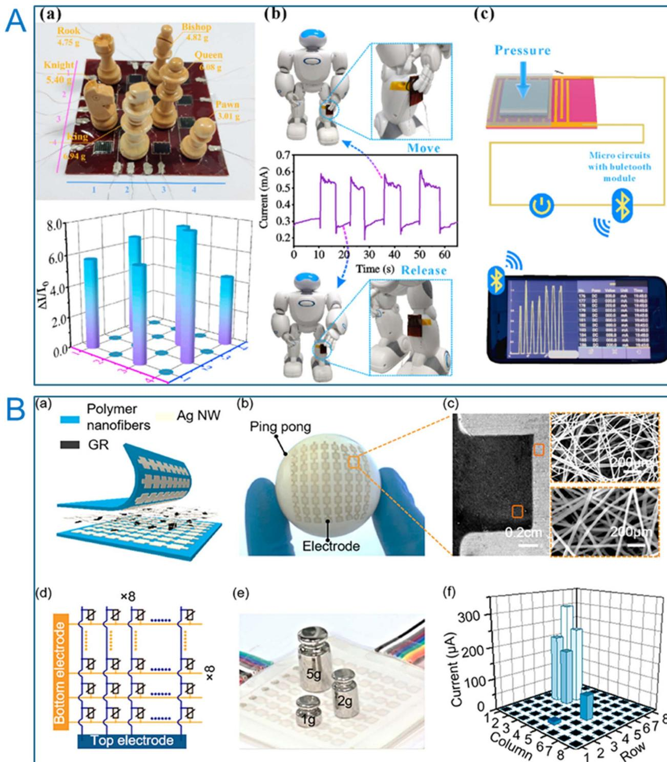
Fig. 3 (A) Flexible pressure sensor for array pressure distribution and human–robot interaction.<sup>27</sup> (B) Fiber electronics for pressure detection and learning in table tennis.<sup>28</sup>
