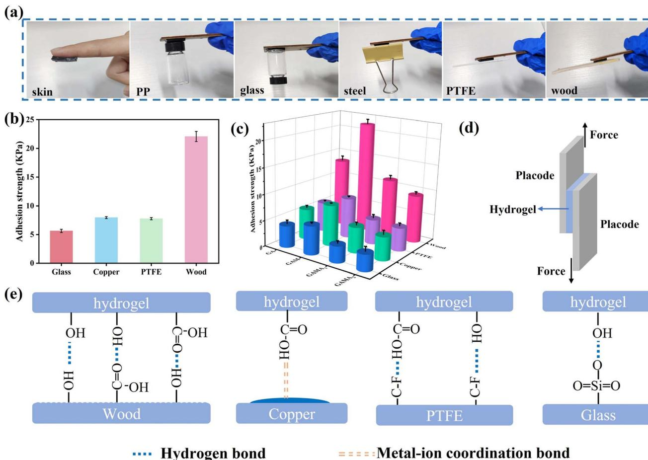
Fig. 4 Adhesion properties of hydrogels. (a) Adhesive performance of the GAMA<sub>2</sub> hydrogel to various substrate surfaces at room temperature. (b) The adhesion strength of GAM hydrogel to various substrates. (c) The adhesion strength of hydrogels with different conductive fillers to different substrates. (d) Schematic of the lap shear test. (e) Adhesion mechanisms to various substrates.
