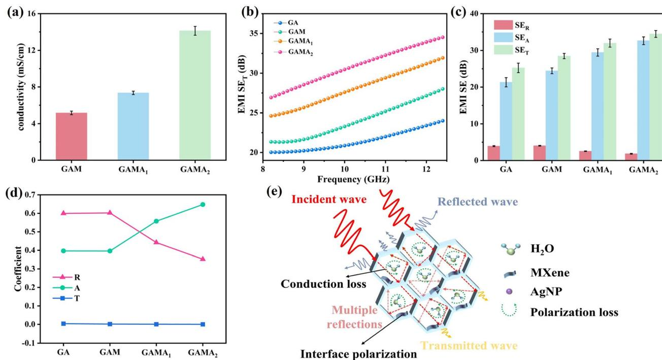
Fig. 5 EMI shielding performance of hydrogels. (a) Electrical conductivity of hydrogels. (b) EMI  $SE_T$  of different hydrogels in the frequency range of 8.2–12.4 GHz. (c) The  $SE_R$ ,  $SE_A$ , and  $SE_T$  of different hydrogels at 12.4 GHz. (d)  $R$ – $A$ – $T$  coefficients of different hydrogels. (e) Scheme showing the EMI shielding mechanism.
