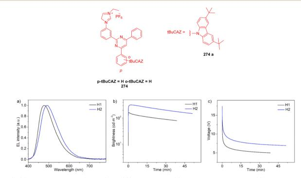
Fig. 116 (top) Chemical structure of tBuCAZ and (bottom) (a) peak EL intensity, (b) time-dependent brightness and (c) time-dependent voltage. Adapted from ref. 336 with permission from Elsevier, Copyright © 2022.
