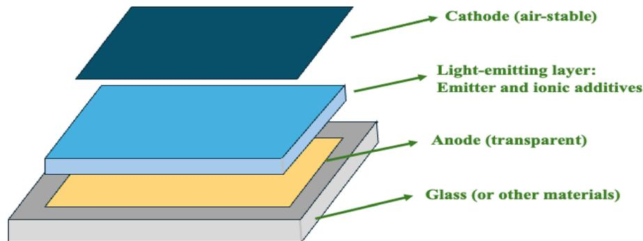
Fig. 109 Schematic diagram of a general LEEC device.
