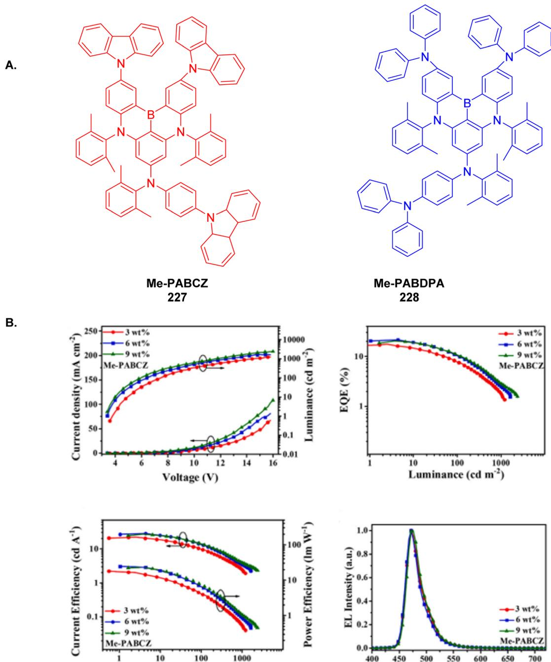
Fig. 77 (A) Chemical structures of PAB, Me-PABCZ, and Me-PABDPA (B) EL characteristics of Me-PABCZ based OLEDs using different doping concentrations: current  $J$ - $V$ - $L$  characteristics; EQE-luminance curves; current efficiency-luminance-power efficiency curves; normalized EL spectra at 6 V.
