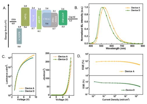
Fig. 81 (A) Device structure and energy level diagram. (B) EL spectra of devices A and D. (C) Luminance–voltage, current density–voltage, and (D) EQE–current density curves of devices A and D.
