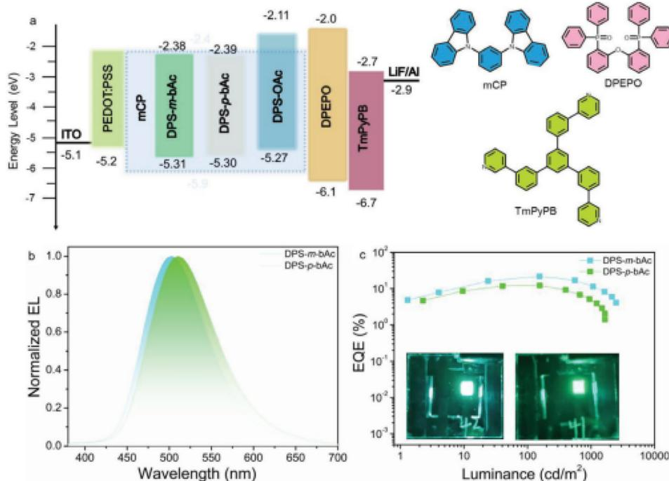
Fig. 87 The energy levels, molecular structures in the device, and device performance. (a) energy levels of the device; (b) molecular structures; (c) EL spectra of the devices; (d) EQE–current density curves. (Inset) The images of the devices (left is DPS-*m*-bAc, and right is DPS-*p*-bAc).
