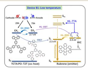
Fig. 95 Diagram showing room-temperature energy transfer mechanisms in device B1 without a CzDBA sensitizer. Schematic illustration of low-temperature energy transfer mechanisms in device B1 without a CzDBA sensitizer. Adapted from ref. 299, with the permission of AIP Publishing.
