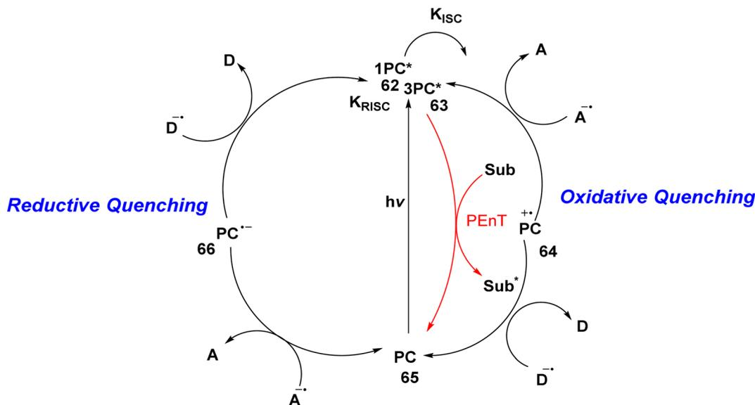
Fig. 43 Photocatalytic cycles of a typical PC with general donor D and acceptor A. Reproduced from ref. 208, <https://doi.org/10.1039/D1CS00198A>, under the terms of the CC BY-NC 3.0 license, <https://creativecommons.org/licenses/by-nc/3.0/>.
