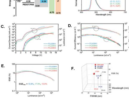
Fig. 83 Chemical structure of (A) device architecture and energy level diagram of the prepared OLEDs (B) current density *versus* voltage, (C) luminance *versus* voltage, and (D) current efficiency–luminance–power efficiency characteristics (CE–L–PE) (E) external quantum efficiency luminance plots (F) summary of the EQE *versus* EL peak wavelength and FWHM plots for the reported narrowband emissive TADF polymer OLEDs.
