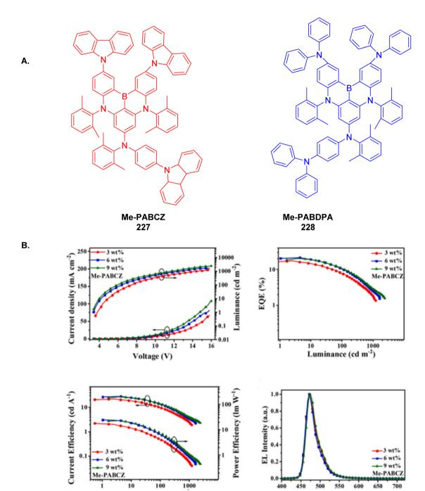
Fig. 77 (A) Chemical structures of PAB, Me-PABCZ, and Me-PABDPA (B) EL characteristics of Me-PABCZ based OLEDs using different doping concentrations: current J-V-L characteristics; EQE-luminance curves; current efficiency-luminance-power efficiency curves; normalized EL spectra at 6 V.
