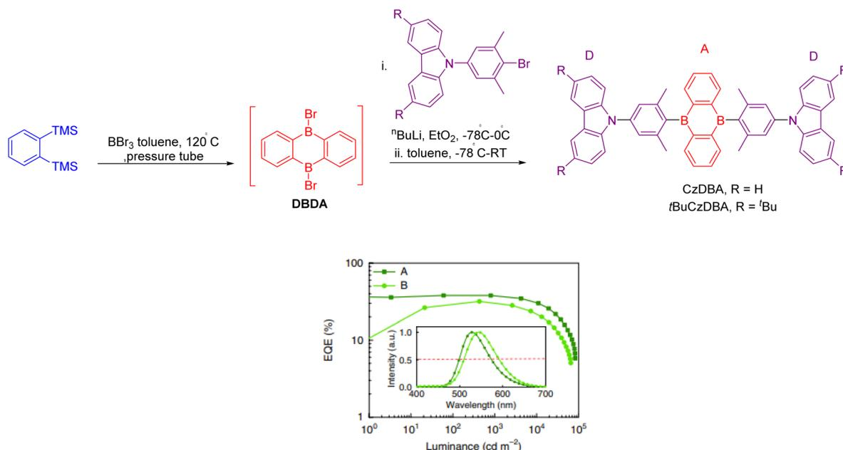
Fig. 79 Synthetic route of CzDBA and tBuCzDBA and along with external quantum efficiency versus luminance electroluminescent spectra.<sup>270</sup>
