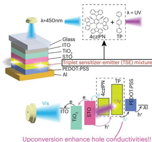
Fig. 98 Visible light-assisted charge extraction in high bandgap  $\text{SrTiO}_3$  through the integration of triplet sensitizer-emitter thin film. Reproduced from ref. 302 with permission from American Chemical Society, Copyright © 2024.
