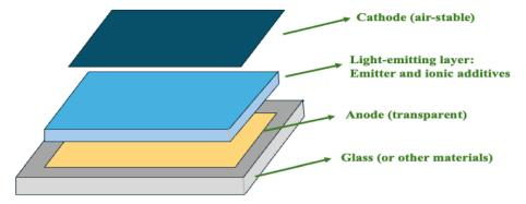
Fig. 109 Schematic diagram of a general LEEC device.
