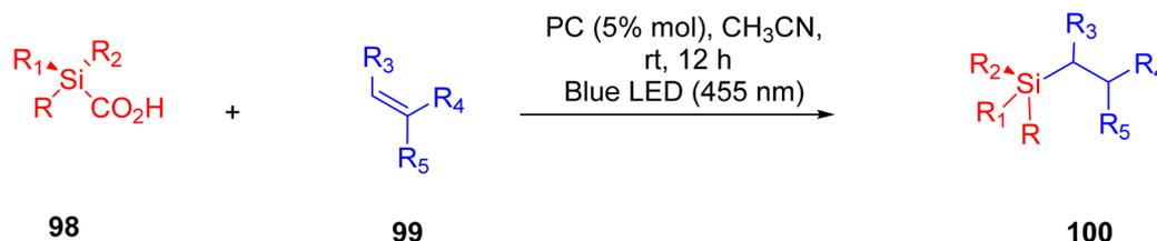
Fig. 55 Hydrosilylation of alkene.<sup>237</sup>
