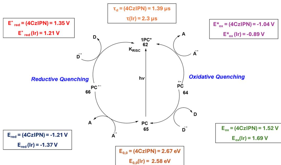
Fig. 47 Photocatalytic cycle comparison of redox and photophysical properties of 4CzIPN. Adapted from ref. 208, <https://doi.org/10.1039/D1CS00198A>, under the terms of the CC BY-NC 3.0 license, <https://creativecommons.org/licenses/by-nc/3.0/>.
