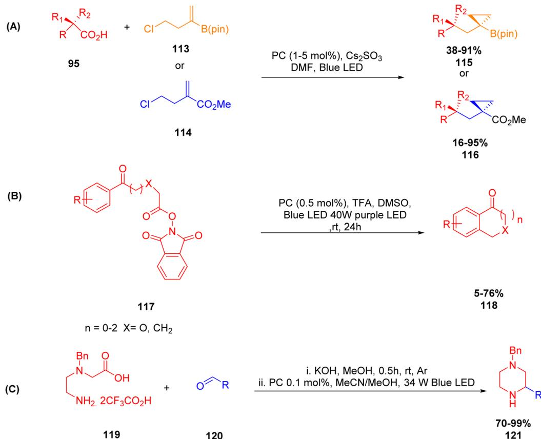
Fig. 60 Schemes for cyclization reactions involving photoinduced decarboxylation mechanism used to synthesize (A) functionalized cyclopropanes,<sup>242</sup> (B) synthesis of intramolecularly alkylated arenes<sup>243</sup> and (C) synthesis of 2-substituted piperazines.<sup>244</sup>
