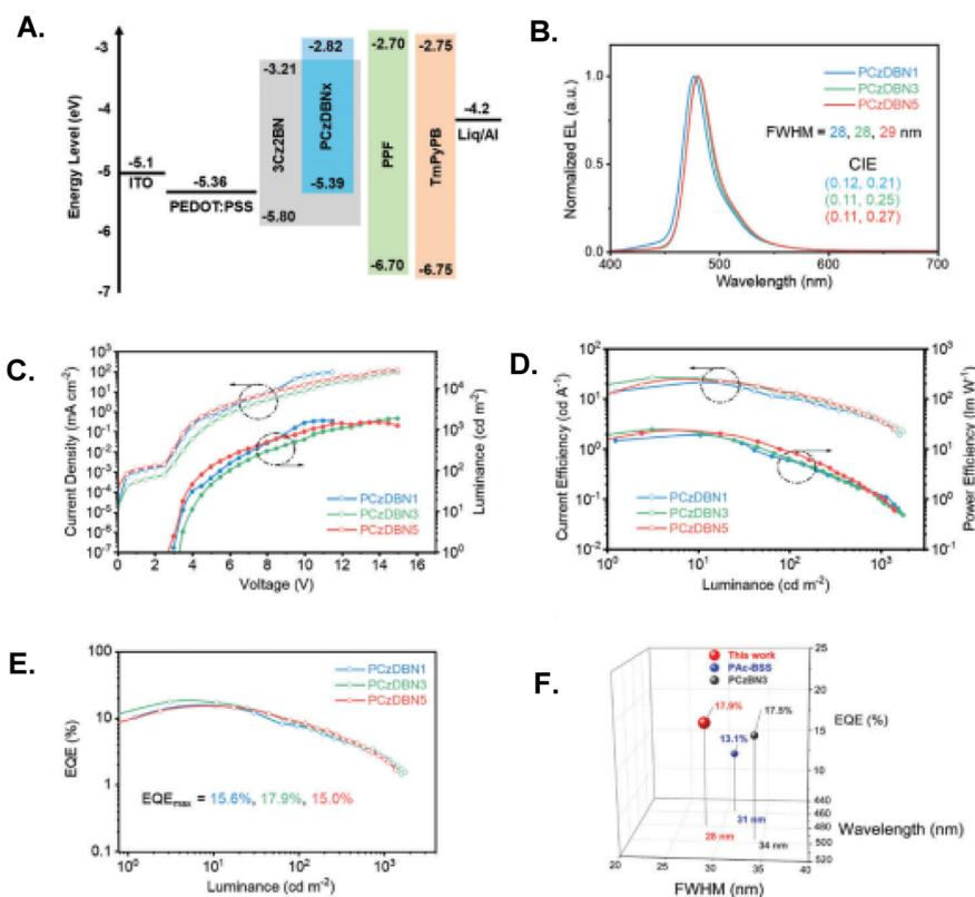
**Fig. 83** Chemical structure of (A) device architecture and energy level diagram of the prepared OLEDs (B) current density versus voltage, (C) luminance versus voltage, and (D) current efficiency–luminance–power efficiency characteristics (CE–L–PE) (E) external quantum efficiency luminance plots (F) summary of the EQE versus EL peak wavelength and FWHM plots for the reported narrowband emissive TADF polymer OLEDs.
