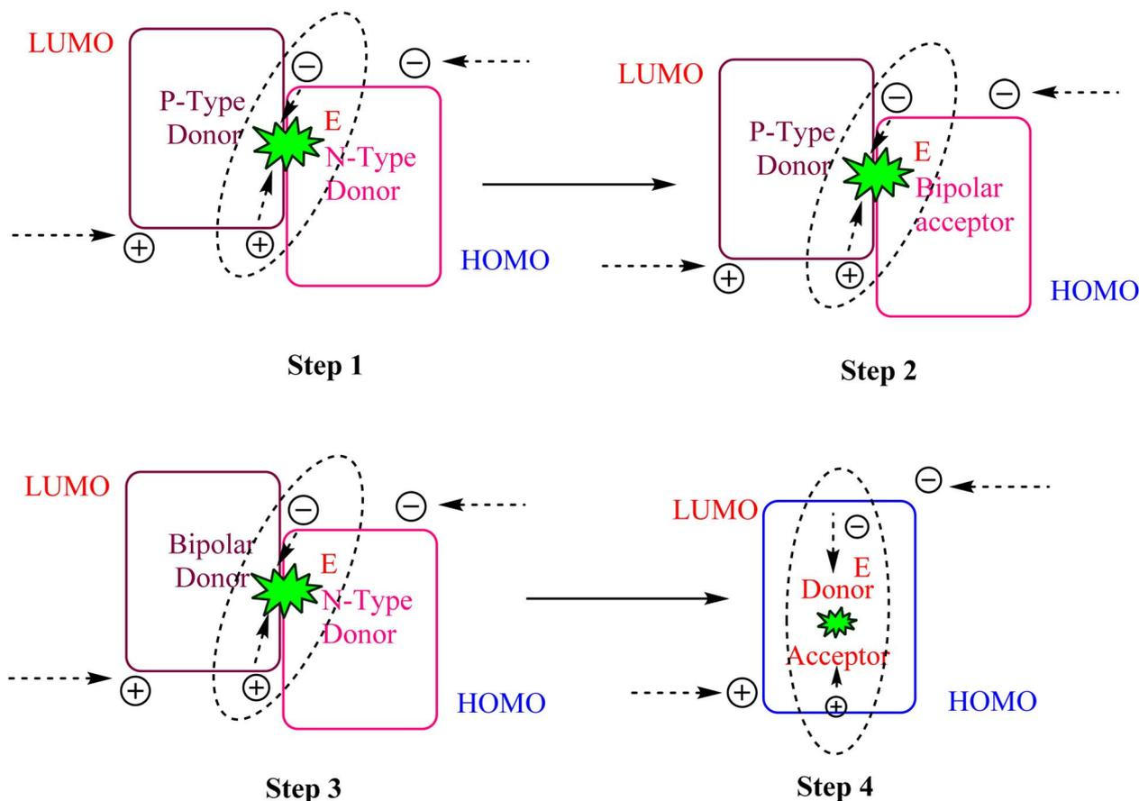
Fig. 4 Mechanism for generation of exciplexes by co-doping.
