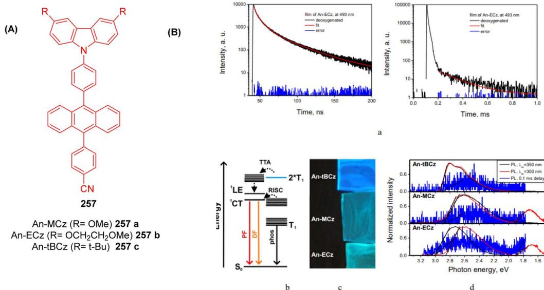
Fig. 96 (A) Molecular structure of An-MCz (257a), An-MCz (257b), and An-tBCz (257c) (B) (a) PL decay curves of the films (b) diagram illustrating the electronic states and transitions of the molecules (c) a photograph of the films of the compounds produced by deposition on drop casting on FTO substrates (d) PL spectra with varying delays. Reproduced from ref. 273, <https://doi.org/10.1021/acsaelm.4c00533>, under the terms of the CC BY 4.0 license, <https://creativecommons.org/licenses/by/4.0/>.
