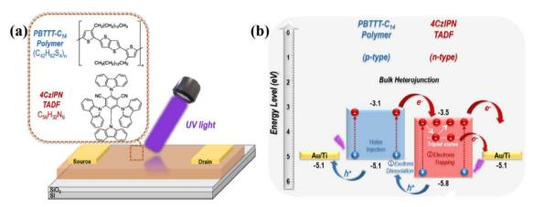
Fig. 101 (a) Diagram of the device structure and (b) energy level diagram in PBTTT-C14 polymer and 4CzIPN bulk heterojunction photo-transistor. Reproduced from ref. 305 with permission from John Wiley & Sons, Copyright © 2024, Wiley-VCH Verlag GmbH & Co. KGaA, Weinheim
