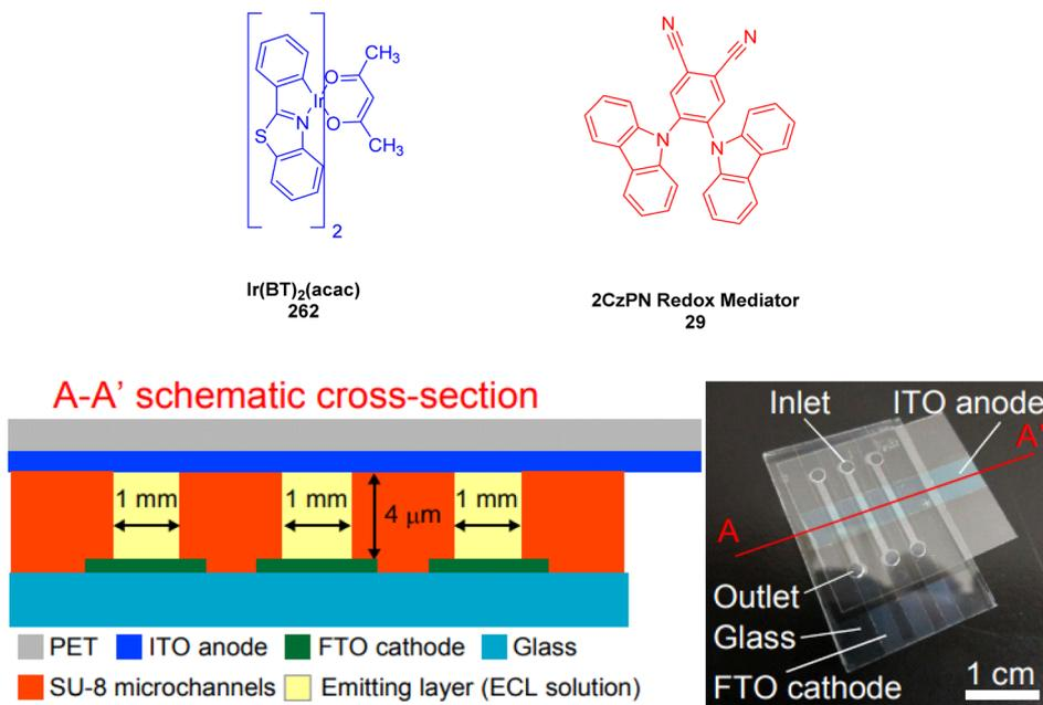
Fig. 104 Molecular representation of 2CzPN (29) and Ir(BT)<sub>2</sub>(acac) (262) along with the microfluidic ECL cell with a schematic cross-section. Reproduced from ref. 309, <https://doi.org/10.5796/electrochemistry.23-00147>, under the terms of the CC BY 4.0 license, <https://creativecommons.org/licenses/by/4.0/>.
