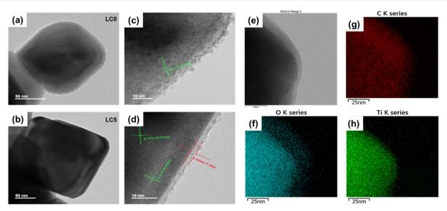
Fig. 5 TEM images of LCO (a and c) and LC5 (b and d). (e-h) EDX mapping photographs for C, Si, and O in sample LC5.
