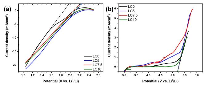
Fig. 8 Catalytic performances of LC0, LC5, LC7.5, and LC10. (a) HER and (b) OER polarization curves measured in  $0.1 \,\mathrm{M}\,\mathrm{Na}_2\mathrm{SO}_4$  aqueous solution for different samples. All measured voltages were converted to values  $v\mathrm{s}$ . Li $^+$ /Li.
