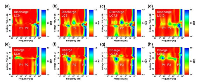
Fig. 9 Color-mapped DRT plots showing Li transition paths for the LC0, LC5, LC7.5, and LC10 electrodes during (a-d) lithiation and (e-h) delithiation.
