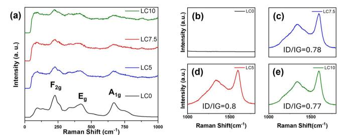
Fig. 3 (a) Raman spectra of LC0, LC5, LC5, LC5, and LC10, covering the  $0-1000\,\mathrm{cm}^{-1}$  range. (b-d) Zoomed-in view of the  $1000-1800\,\mathrm{cm}^{-1}$  region, showing the D-band and G-band characteristics of all samples.
