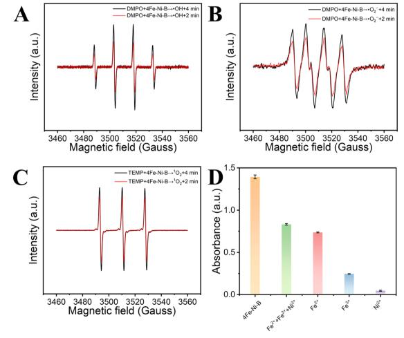
Fig. 4 EPR spectra of DMPO spin trapping in the solution of 'OH and 'O<sub>2</sub><sup>-</sup> (A) and (B); EPR spectrum of TEMP spin trapping in the solution of  $^{1}O_{2}$  (C); comparison of peroxidase activities of 4Fe-Ni-B, Fe<sup>2+</sup> + Fe<sup>3+</sup> + Ni<sup>2+</sup>, Fe<sup>2+</sup>, Fe<sup>3+</sup> and Ni<sup>2+</sup>, and ion concentrations were the same as those in the ICP experiment (D).
