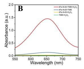
Fig. 3 UV-Vis absorption spectra of the oxidized TMB in different systems: (A) different nanozymes; (B)  $4Fe-Ni-B+TMB+H_2O_2$ ; 4Fe-Ni-B+TMB;  $4Fe-Ni-B+H_2O_2$ ; and  $TMB+H_2O_2$ .
