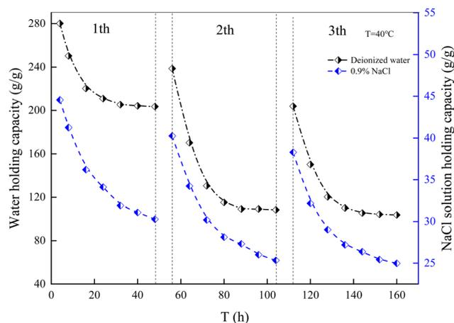
**Fig. 4** Reswelling and water holding ability of WS/PAA–PAM.
