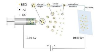
**Fig. 2** Schematic of RDX/Al/NC composite explosive preparation *via* electrostatic spraying.
