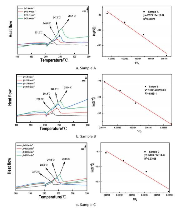
Fig. 10 DSC and fitting curves of sample A (a), sample B (b) and sample C (c) at different heating rates.
