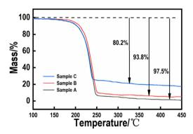
Fig. 9  $\,$  TG curves of RDX/Al/NC composite explosives at a heating rate of 10 K min $^{-1}$ .
