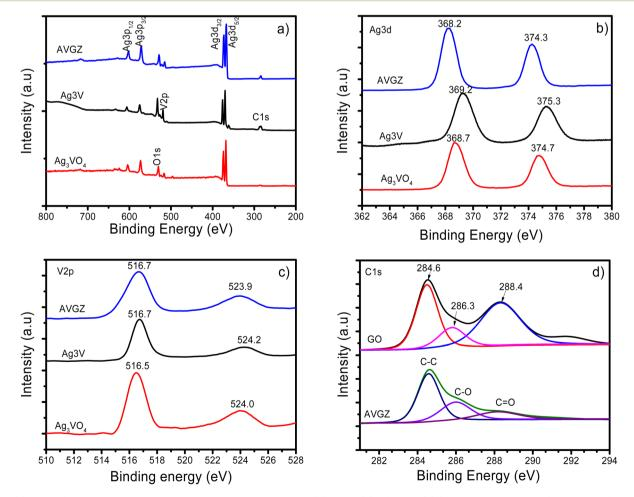
Fig. 4 (a) The XPS scan with the respective high-resolution spectra of (b) Ag 3d, (c) V 2p, and (d) C 1s core level of Ag<sub>3</sub>VO<sub>4</sub>, Ag<sub>3</sub>V, AVGZ and GO catalysts.
