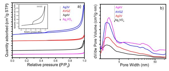
Fig. 3 Nitrogen adsorption-desorption isotherms at 77 K (a) and pore size distribution (b) of the materials.
