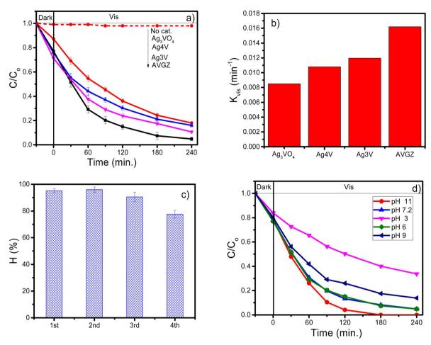
Fig. 6 DDT degradation process on catalysts (a), reaction rate constants (b), catalyst reusability of AVGZ (c), and the effect of pH on the reaction process (d).
