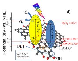
Fig. 9 The effect of oxidation inhibitors (a), spin trapping of  $\cdot O_2^-$  and  $\cdot OH$  with DMPO (b and c), and the proposed mechanism for the degradation of DDT on AVGZ (d).
