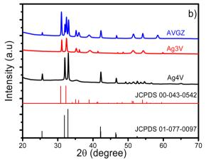
Fig. 1 XRD patterns of GO (a), Ag<sub>3</sub>VO<sub>4</sub> (a), Ag<sub>3</sub>V (a and b), Ag<sub>4</sub>V (b), and AVGZ (b).
