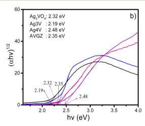
Fig. 5 UV-Vis absorption spectra (a) and  $E_{bq}$  calculation (b) using the Kubelka-Munk method (K-M) of Ag<sub>3</sub>VO<sub>4</sub>, Ag3V, Ag4V, and AVGZ.
