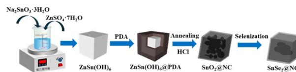
Fig. 1 Schematic of formation process of Cube SnSe<sub>2</sub>@NC.
