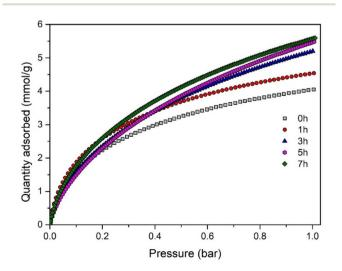
CO<sub>2</sub> adsorption isotherms at 0 °C for different activation times.
