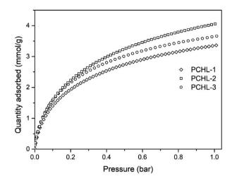
Fig. 3 CO<sub>2</sub> adsorption isotherms at 0 °C of chitosan-based porous carbon monoliths.
