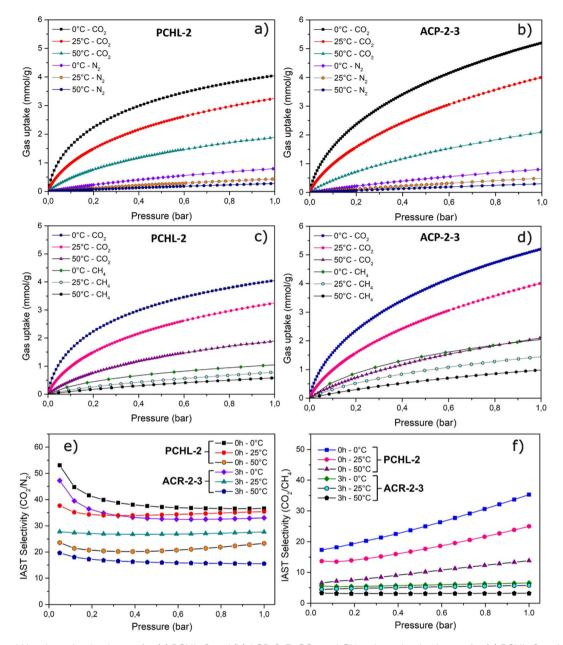
Fig. 7  $CO_2$  and  $N_2$  adsorption isotherms for (a) PCHL-2 and (b) ACP-2-3;  $CO_2$  and  $CH_4$  adsorption isotherms for (c) PCHL-2 and (d) ACP-2-3; IAST selectivity analyses for (e) (15 : 85)  $CO_2/N_2$  mixture and (f) (50 : 50)  $CO_2/CH_4$  mixture, for PCHL-2 (t=0 h) and ACP-2-3 (t=3 h).
