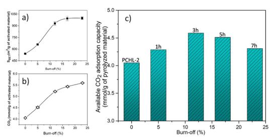
Fig. 6 Evolution of the (a) BET surface area, (b)  $CO_2$  uptake (at 0 °C and 1 bar), and (c) available  $CO_2$  adsorption capacity of the activated carbons with burn-off.
