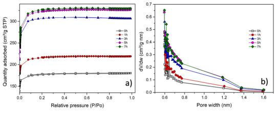
(a) N<sub>2</sub> sorption isotherms for different activation times. (b) Pore size distributions (PSDs) calculated from the Horvath-Kawazoe method.
