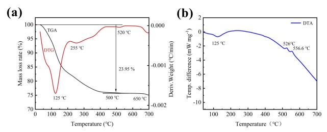
Fig. 3 TGA/DTG (a) and DTA (b) curves of the initial sample.
