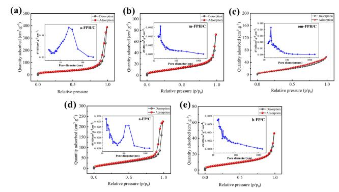
N<sub>2</sub> adsorption-desorption isotherm and pore size distribution of a-FPH/C (a), m-FPH/C (b), om-FPH/C (c), a-FP/C (d), and h-FP/C (e).
