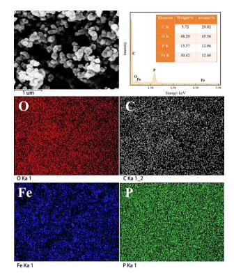
Fig. 7 Element distribution mappings of a-FPH/C.
