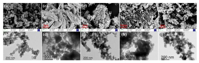
Fig. 6 SEM and TEM of samples. (a) and (b) are SEM and TEM of a-FPH/C, (c) and (d) are SEM and TEM of m-FPH/C, (e) and (f) are SEM and TEM of om-FPH/C, (g) and (h) are SEM and TEM of a-FP/C, (i) and (j) are SEM and TEM of h-FP/C.
