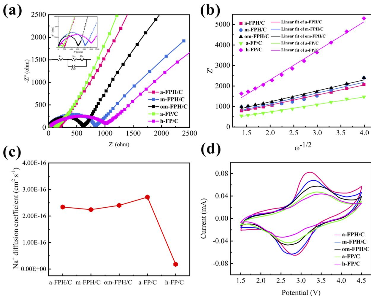
Fig. 9 Electrochemical impedance spectroscopy of samples (a). The relationship between the resistance ( $Z'$ ) and the inverse square root of the angular speed (b). The slope ( $\delta$ ) and  $\text{Na}^+$  diffusion coefficient of samples (c). Cyclic voltammetry of samples at a scan rate of  $0.1 \text{ mV s}^{-1}$  in the voltage range of 1.5–4.5 V at room temperature (d).
