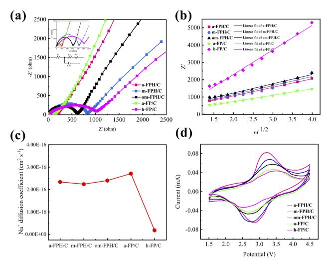
Fig. 9 Electrochemical impedance spectroscopy of samples (a). The relationship between the resistance (Z') and the inverse square root of the angular speed (b). The slope ( $\delta$ ) and Na<sup>+</sup> diffusion coefficient of samples (c). Cyclic voltammetry of samples at a scan rate of 0.1 mV s<sup>-1</sup> in the voltage range of 1.5–4.5 V at room temperature (d).
