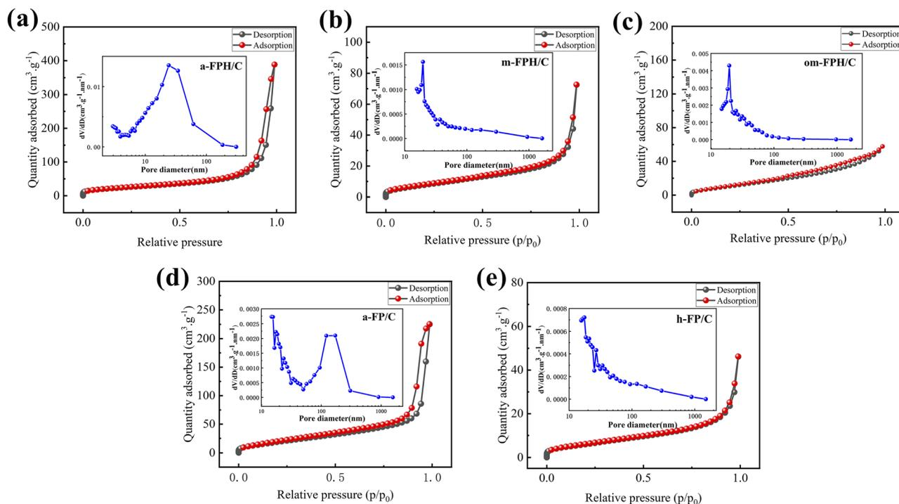
Fig. 8  $N_2$  adsorption–desorption isotherm and pore size distribution of a-FPH/C (a), m-FPH/C (b), om-FPH/C (c), a-FP/C (d), and h-FP/C (e).
