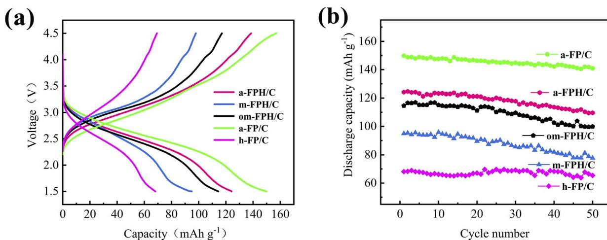
Fig. 10 Charge-discharge curves (a) of samples and cycling performance (b) of samples at 0.1C at room temperature.
