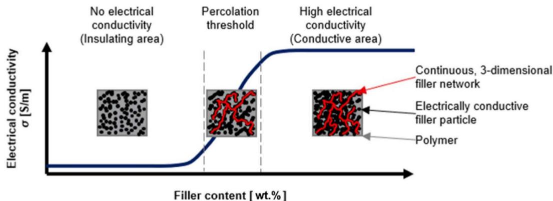
Fig. 5 The mechanism of electrical conductivity in polymer nanocomposites depending on the amount of introduced filler.<sup>132</sup>
