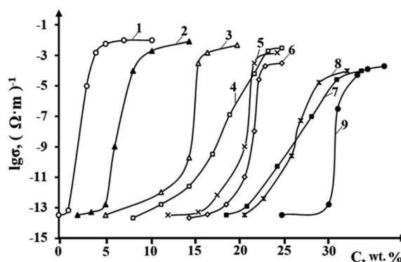
Fig. 10 Effect of the content of different grades of CB on the electrical conductivity of HDPE-based composites: (1) – Printex XE 2B; (2) – acetylene soot; (3) – N-550; (4) – P-514; (5) – P-324; (6) – P-803; (7) – K-354; (8) – P-234; (9) – T-900.<sup>158</sup>
