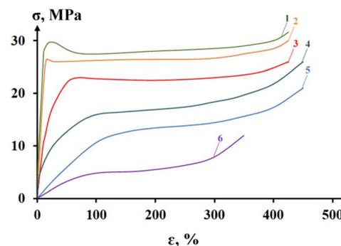
Fig. 11 Effect of the content of the elastomer component on the stress–strain curves of polymer blends based on compatibilized HDPE + SCS-30, wt%: (1) – initial HDPE; (2) – 10; (3) – 20; (4) – 30; (5) – 40; (6) – 50.<sup>183</sup>
