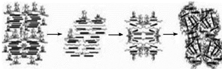
Fig. 2 Scheme of polymer nanocomposite formation.<sup>38</sup>
