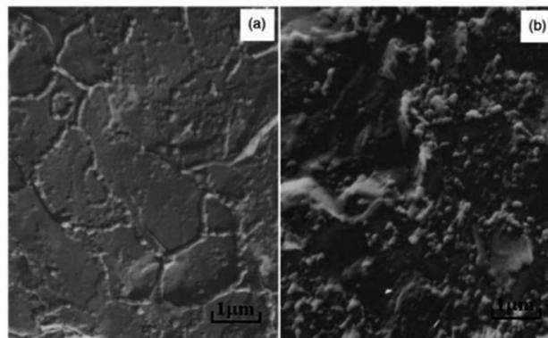
Fig. 6 Electron microscopic images of HDPE + 5.0 wt% CB (a) and HDPE + 20 wt% CB (b) nanocomposites. Magnification  $\times 15\,000$ .<sup>143</sup>
