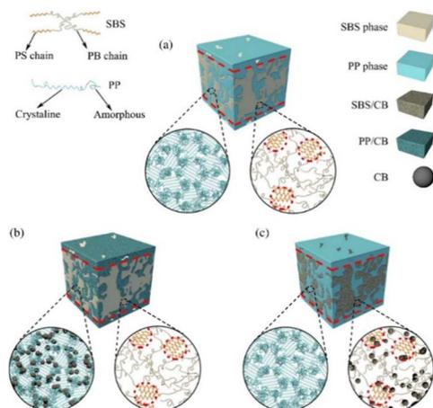
Fig. 9 Schematic representation of the distribution of CB in various forms: (a) without CB, (b) CB in PP, (c) CB in SBS.<sup>156</sup>
