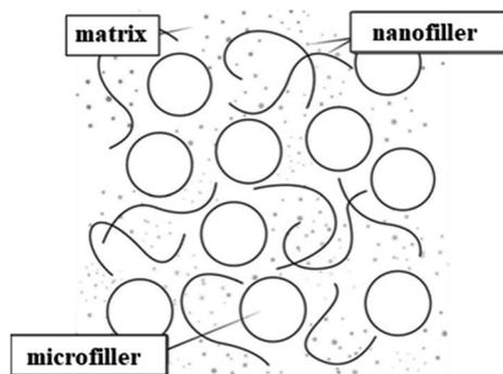
Fig. 1 Morphology of micro- and nanofilled composites.<sup>32</sup>
