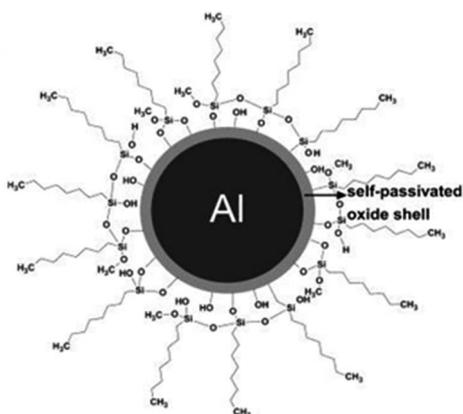
Fig. 4 Schematic representation of surface-modified aluminum nanoparticles.<sup>104</sup>
