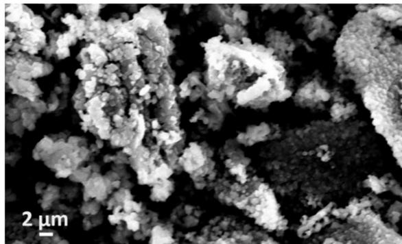
Fig. 8 SEM image of Fe<sub>3</sub>O<sub>4</sub> used to evaluate biological inhibition.
