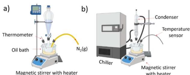
Fig. 2 Schematic representation of the apparatus for Fe<sub>3</sub>O<sub>4</sub> synthesis using the coprecipitation (a) and polyol (b) methods.
