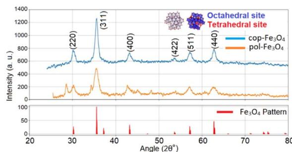
Fig. 5  $\text{Fe}_3\text{O}_4$  pattern, cop- $\text{Fe}_3\text{O}_4$  and pol- $\text{Fe}_3\text{O}_4$  X-ray diffractograms.
