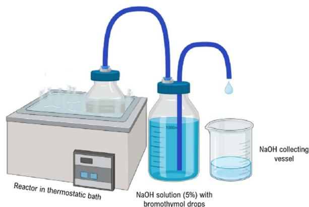
Fig. 3 Schematic representation of the MAT system mounted.
