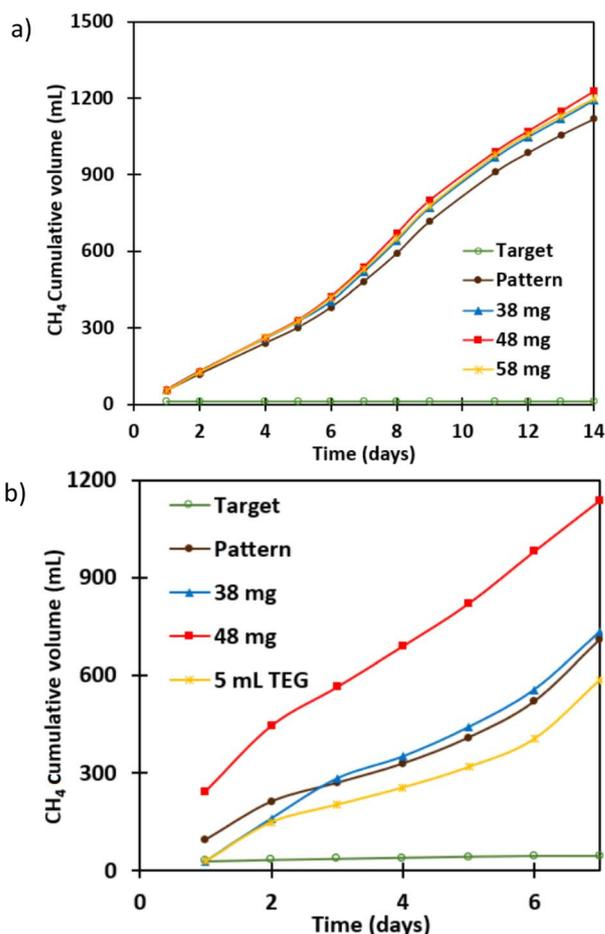
Fig. 6 Total CH<sub>4</sub> production using (a) cop-Fe<sub>3</sub>O<sub>4</sub> (mg) and (b) pol-Fe<sub>3</sub>O<sub>4</sub> (mg) groups.
