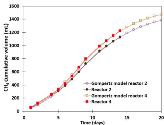
Fig. 7 Gompertz model to reactors 2 and 4 of enhanced CH<sub>4</sub> production with cop-Fe<sub>3</sub>O<sub>4</sub>.
