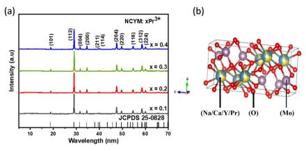
Fig. 1 (a) XRD of the NCYM: $xPr^{3+}$  (x = 0.1, 0.2, 0.3 and 0.4), (b) crystal structure of NCYM.
