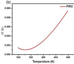
Fig. 9 (a and b) Temperature resolution values  $\delta T$ , corresponding to (a) FIR<sub>2</sub> ( $^{3}P_{1} - ^{3}H_{5}/^{3}P_{0} - ^{3}H_{5}$ ) and (b) FIR<sub>3</sub> ( $^{3}P_{1} - ^{3}H_{5}/^{3}P_{0} - ^{3}F_{2}$ ) for NCYM:0.3Pr<sup>3+</sup>.
