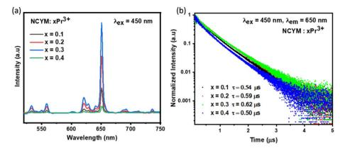
Fig. 5 (a) Emission spectrum of NCYM:xPr $^{3+}$  (x = 0.1, 0.2, 0.3 and 0.4) excited at 450 nm, (b) decay curves of the 650 nm emission for the samples with different Pr $^{3+}$  concentrations under 450 nm excitation.
