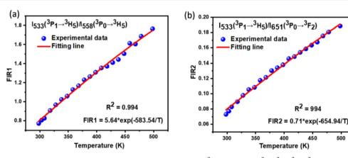
Fig. 7 (a and b) Variations of FIR as a function of temperature for NCYM:0.3Pr<sup>3+</sup> between (a)  $(^{3}P_{1} - ^{3}H_{5})^{7}P_{0} - ^{3}H_{5})$ , and (b)  $(^{3}P_{1} - ^{3}H_{5})^{7}P_{0} - ^{3}F_{2})$ .
