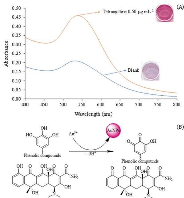
Fig. 1 Gold nanoparticle formation induced by natural phenolic compounds, (A) surface plasmon resonance (SPR) of gold nanoparticles and (B) a possible reaction path.
