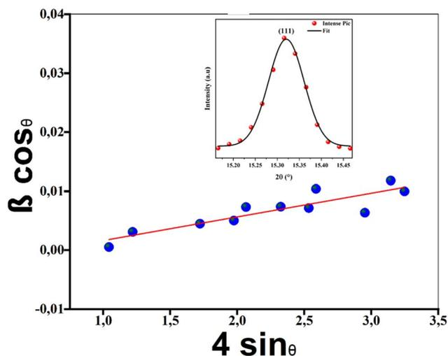
Fig. 3 The strain graph, (the Debye–Scherrer plot for  $K_2SnCl_6$  compound shown inset).
