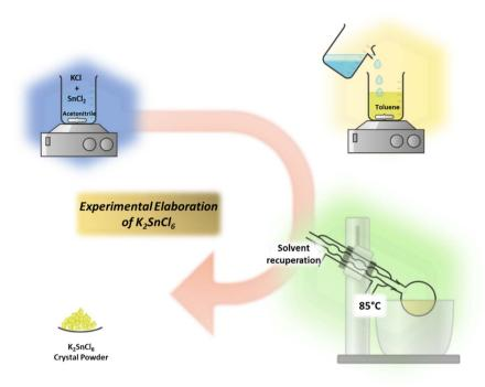
Fig. 1 A schematic representation of the antisolvant method to obtain K<sub>2</sub>SnCl<sub>6</sub> single crystals.
