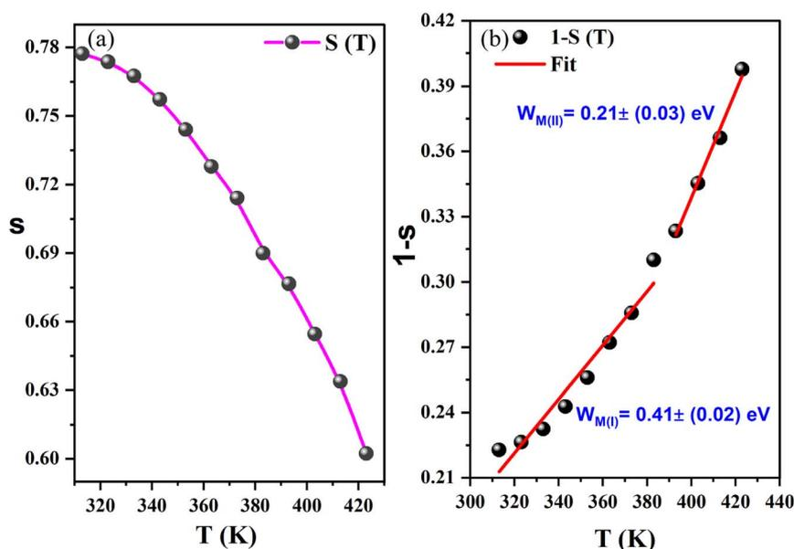
Fig. 10 (a) The temperature dependence of the frequency exponent  $s$ , (b): evolution of  $(1 - s)$  against the temperature and the deduced  $W_M^{(I)}$  and  $W_M^{(II)}$  energies for the CBH mechanism.
