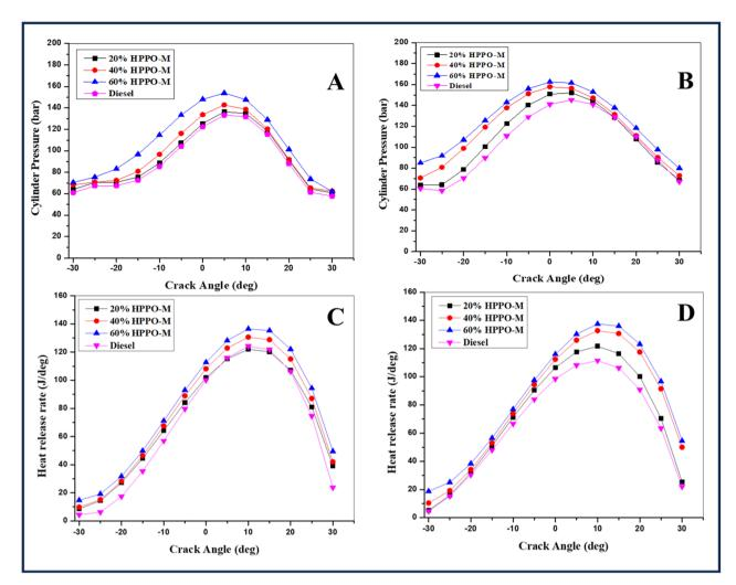
Cylinder pressure variation for (A) 100% load and (B) 75% load and variations in heating release rate (HRR) for (C) 100% load and (D) 75% load
