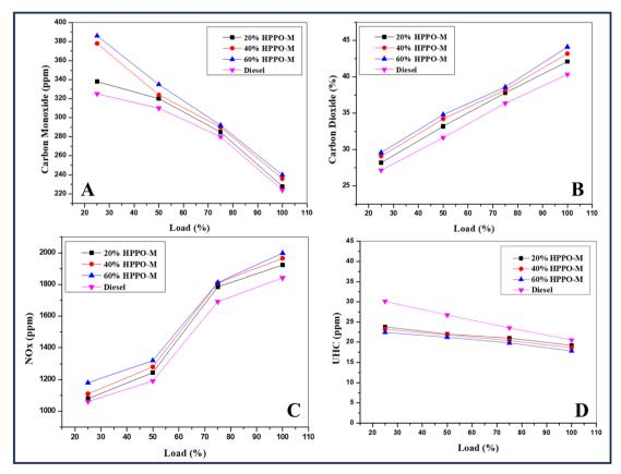
Fig. 8 Variation of (A) CO with load, (B) CO<sub>2</sub> with load, (C) NOx with load and (D) HC with load.
