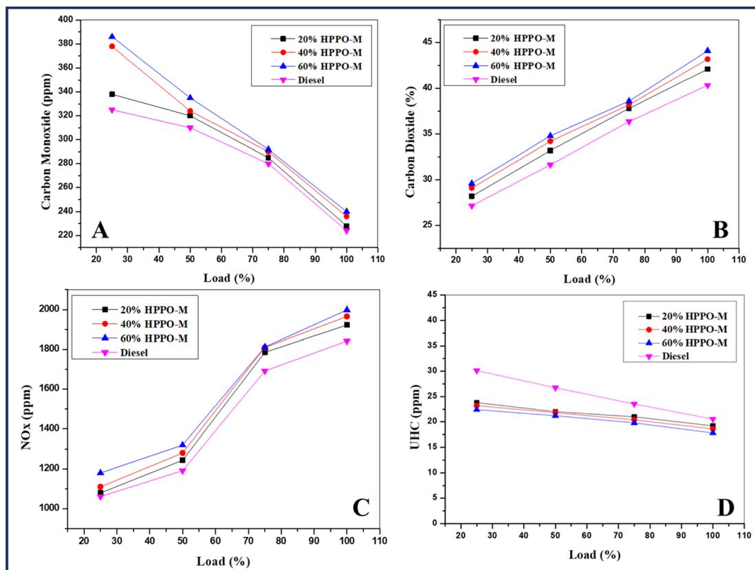
Fig. 8 Variation of (A) CO with load, (B) CO<sub>2</sub> with load, (C) NOx with load and (D) HC with load.
