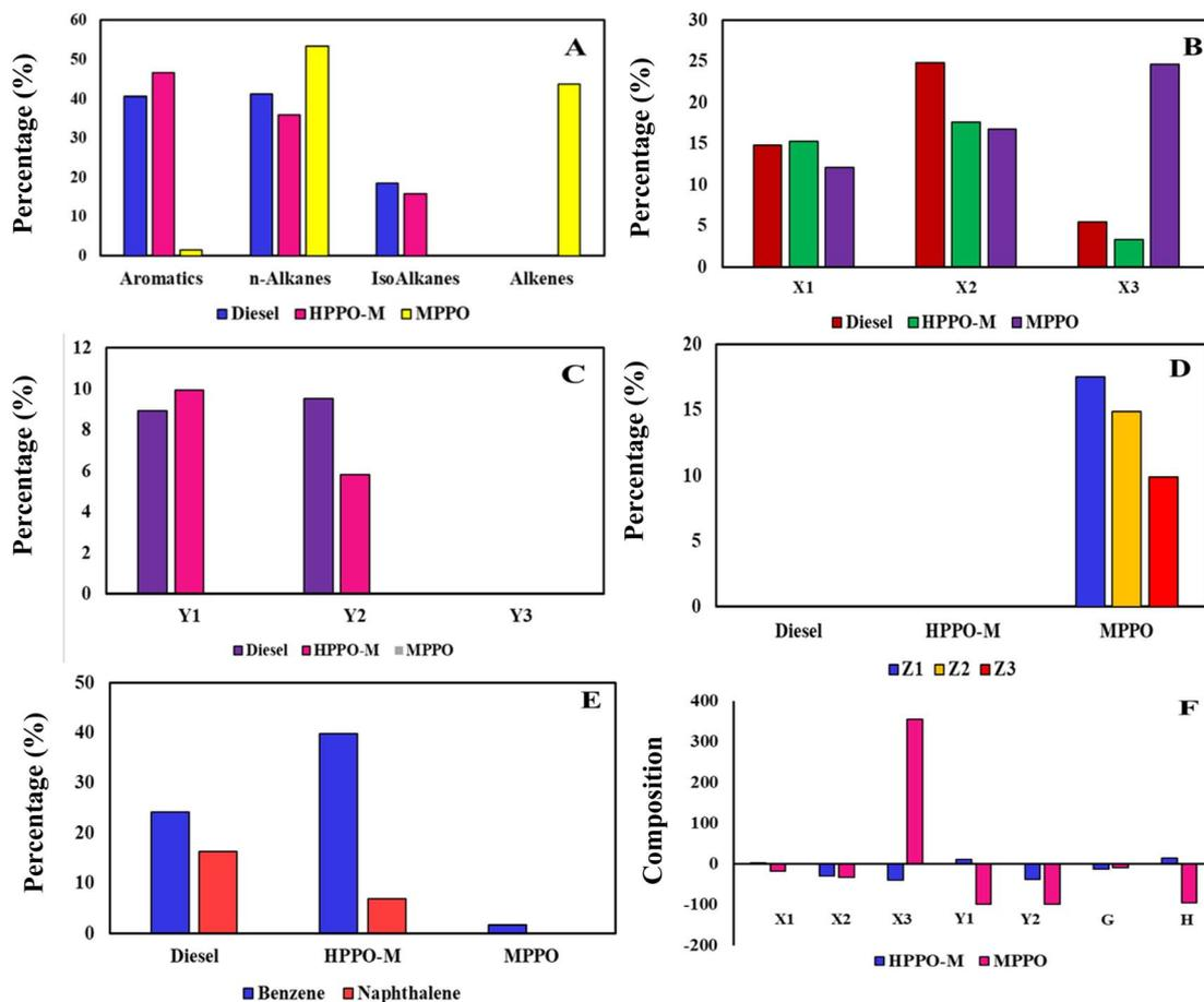
Fig. 5 (A) Fuel composition of diesel, HPPO-M, and MPPO. Carbon number range of (B) *n*-alkanes in diesel, HPPO-M, and MPPO and (C) isoalkanes in diesel, HPPO-M, and MPPO. (D) Alkenes in diesel, HPPO-M, and MPPO. (E) Aromatic compounds of benzene and naphthalene in diesel, HPPO-M, and MPPO. (F) Percentage variation in the chemical composition of MPPO and HPPO-M with diesel.
