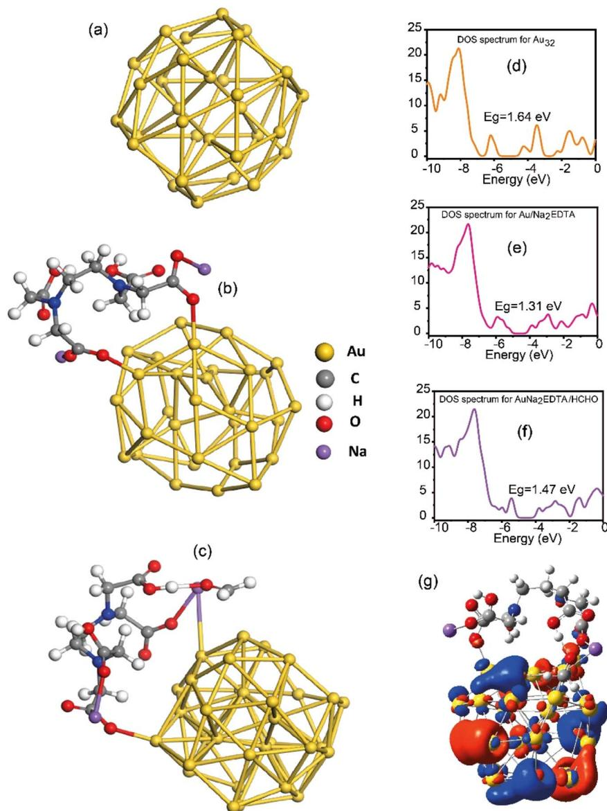
Fig. 3 Optimized structures of (a) golden fullerene  $\text{Au}_{32}$ , (b)  $\text{AuNa}_2\text{EDTA}$ , (c)  $\text{AuNa}_2\text{EDTA-HCHO}$ , and DOS of (d) golden fullerene  $\text{Au}_{32}$ , (e)  $\text{AuNa}_2\text{EDTA}$  and (f)  $\text{AuNa}_2\text{EDTA-HCHO}$ , (g) MEP map of  $\text{AuNa}_2\text{EDTA-HCHO}$ .
