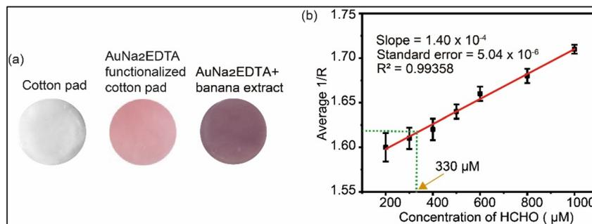
Fig. 6 (a) Photographs taken by smartphone of cotton pad, cotton pad functionalized by AuNa<sub>2</sub>EDTA and incorporation of banana extract on the AuNa<sub>2</sub>EDTA functionalized cotton pad; (b) a calibration curve of average 1/R as a function of formaldehyde concentrations showing the concentration of formaldehyde in banana extract.
