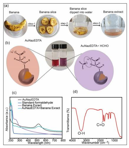
Fig. 5 (a) Stepwise banana extract extraction process; (b) addition of banana extract into AuNa₂EDTA changed solution color from wine red to purplish-blue. Responsible main ingredients for the corresponding color are shown; (c) absorption spectrum of synthesized AuNa<sub>2</sub>EDTA (black), standard formaldehyde (blue), banana extract (purple), after addition of banana extract in AuNa<sub>2</sub>EDTA (green); (d) ATR spectrum of banana extract.
