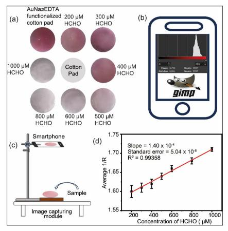
Fig. 4 (a) Photos taken by smartphone of cotton pad, cotton pad functionalized by  $AuNa_2EDTA$  and incorporation of various concentrations of formalin on the  $AuNa_2EDTA$  functionalized cotton pad; (b) illustration of a GIMP software supported smartphone; (c) process of taking photos; (d) a calibration curve of average 1/R as a function of formaldehyde concentrations.
