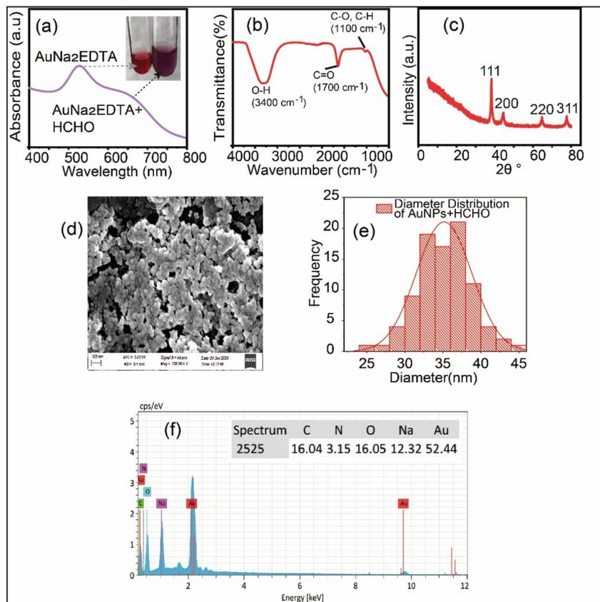
Fig. 2 (a) The UV-vis absorption spectrum of AuNa<sub>2</sub>EDTA–HCHO. Inset shows the solution color after HCHO addition; (b) ATR spectrum of AuNa<sub>2</sub>EDTA–HCHO; (c) the XRD analysis of the AuNPs; (d) SEM image of AuNa<sub>2</sub>EDTA–HCHO; (e) diameter distribution bar chart using ImageJ software; (f) EDX spectrum of AuNa<sub>2</sub>EDTA–HCHO. Inset shows the elemental composition of AuNa<sub>2</sub>EDTA–HCHO.
