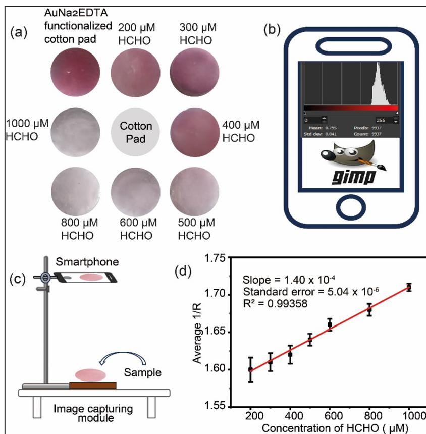
Fig. 4 (a) Photos taken by smartphone of cotton pad, cotton pad functionalized by AuNa<sub>2</sub>EDTA and incorporation of various concentrations of formalin on the AuNa<sub>2</sub>EDTA functionalized cotton pad; (b) illustration of a GIMP software supported smartphone; (c) process of taking photos; (d) a calibration curve of average  $1/R$  as a function of formaldehyde concentrations.
