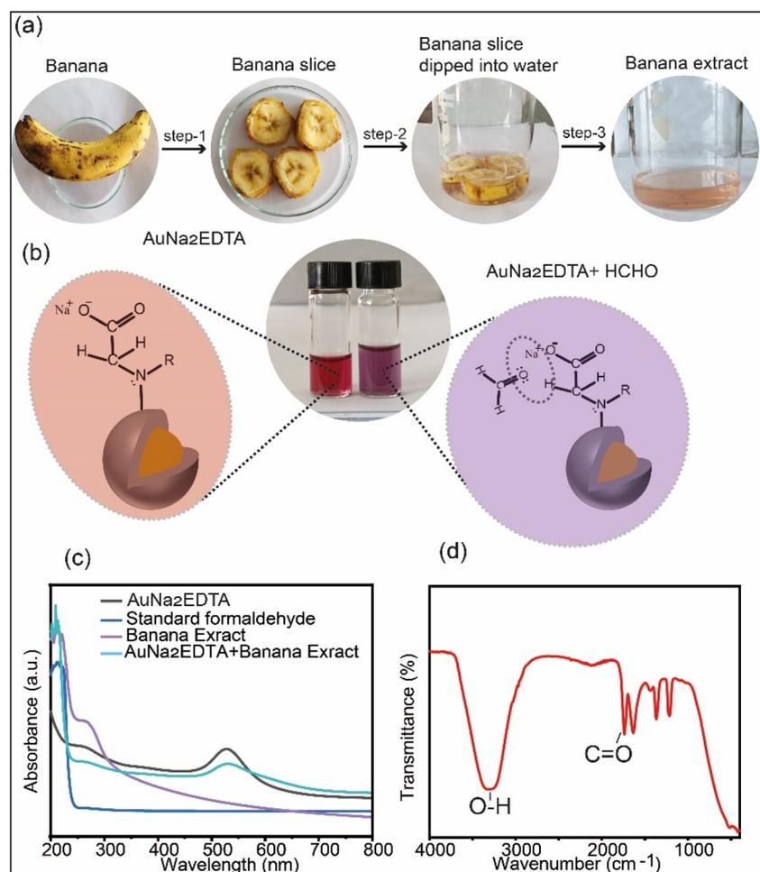
Fig. 5 (a) Stepwise banana extract extraction process; (b) addition of banana extract into  $\text{AuNa}_2\text{EDTA}$  changed solution color from wine red to purplish-blue. Responsible main ingredients for the corresponding color are shown; (c) absorption spectrum of synthesized  $\text{AuNa}_2\text{EDTA}$  (black), standard formaldehyde (blue), banana extract (purple), after addition of banana extract in  $\text{AuNa}_2\text{EDTA}$  (green); (d) ATR spectrum of banana extract.
