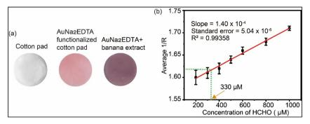
Fig. 6 (a) Photographs taken by smartphone of cotton pad, cotton pad functionalized by  $AuNa_2EDTA$  and incorporation of banana extract on the  $AuNa_2EDTA$  functionalized cotton pad; (b) a calibration curve of average 1/R as a function of formaldehyde concentrations showing the concentration of formaldehyde in banana extract.
