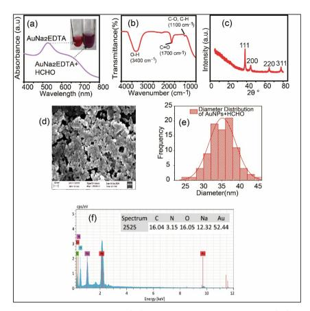
Fig. 2 (a). The UV-vis absorption spectrum of  $AuNa_2EDTA-HCHO$ . Inset shows the solution color after HCHO addition; (b) ATR spectrum of  $AuNa_2EDTA-HCHO$ ; (c) the XRD analysis of the AuNPs; (d) SEM image of  $AuNa_2EDTA-HCHO$ ; (e) diameter distribution bar chart using ImageJ software; (f) EDX spectrum of  $AuNa_2EDTA-HCHO$ . Inset shows the elemental composition of  $AuNa_2EDTA-HCHO$ .
