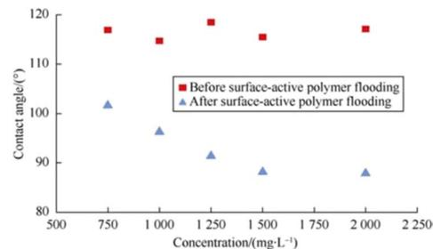
Fig. 19 Change in rock contact angle before and after treatment with surfactant polymers.<sup>96</sup>
