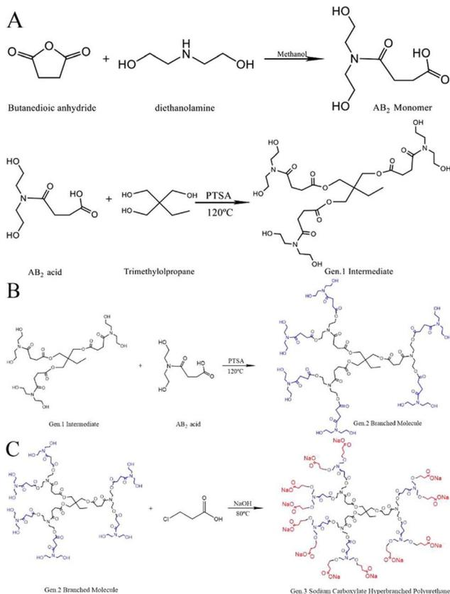
Fig. 16 (A) Synthesis of the AB<sub>2</sub> monomer and Gen.1 intermediate. (B) Synthesis of Gen.2 hyperbranched polyurethane (HPAE). (C) Synthesis of HPAE with sodium carboxylate at the end of Gen.2 (*m*-HPAE).<sup>81</sup>
