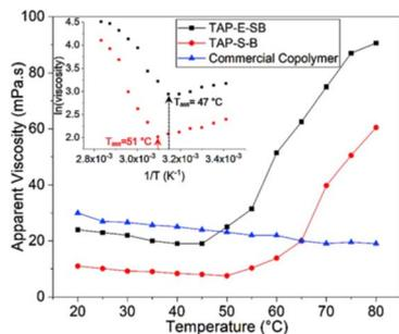
Fig. 18 Viscosity retention of acrylamide-based polymers under high temperature and high salinity conditions. This figure shows the temperature-dependent viscosity behaviour of different acrylamide-based polymers (including TAP-E-SB, TAP-S-B, and commercial AM-based copolymers) at a concentration of 2000 ppm in a 5% KCl aqueous solution.<sup>95</sup>
