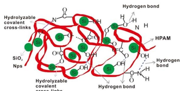
Fig. 14 Potential interactions between SiO<sub>2</sub> and HPAM.<sup>77</sup>
