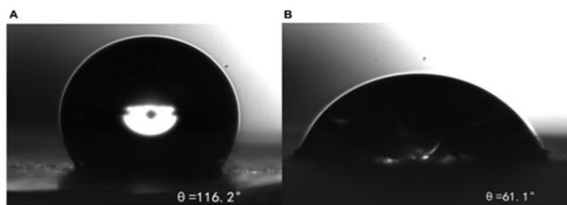
Fig. 17 Contact angle of hydrophobic formation of the rock sample (A) and rock sample after *m*-HPAE treatment (B). This figure demonstrates the interface improvement capability of *m*-HPAE.<sup>81</sup>
