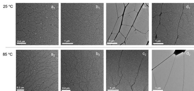
Fig. 20 TEM micrographs for diutan gum (a1 and a2), scleroglucan (b1 and b2), xanthan gum (c1 and c2), and HPAM (d1 and d2) at 25 and 85 °C ( $C_p = 0.05$  wt%, no salt). Diutan gum, scleroglucan, and Xanthan gum were biopolymers produced through fermentation by the bacteria *Sphingomonas*, the plant pathogenic fungus *Sclerotium*, and the bacteria *Xanthomonas*, respectively.<sup>71</sup>
