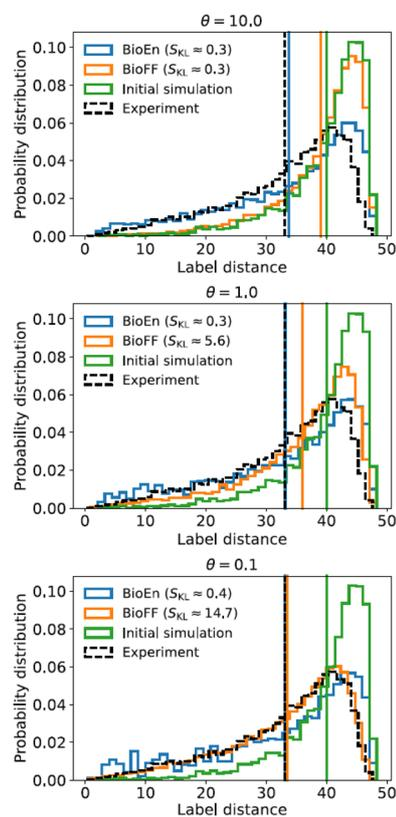
Fig. 4 Prediction of polymer conformational change in saline environments using machine learning-driven force fields. Distribution of the label distance used for refinement and its mean value (vertical lines) for the initial reference simulation ( $\kappa_0 = 20$ , green), the synthetic experimental data ( $\kappa_{\text{exp}} = 10$ , black dashed lines), BioEn (blue), and BioFF (orange). The confidence in the reference ensemble decreases top to bottom ( $\theta = 10, 1, 0.1$ ).<sup>53</sup>
