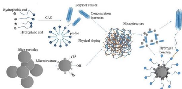
Fig. 13 Mechanism of increasing fluid viscosity by combining silica nanoparticles with amphiphilic polymers.<sup>76</sup>
