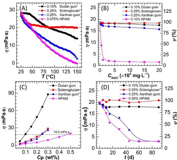
Fig. 8 The viscosity changes of different polymers under different influencing factors. (A) Temperature. (B) Salinity. (C) Polymer concentration. (D) Time.<sup>71</sup>
