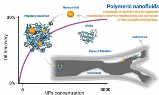
Fig. 15 Macro-micro theoretical mechanism of SiO<sub>2</sub> nanoparticles-polymer flooding system.<sup>78</sup>
