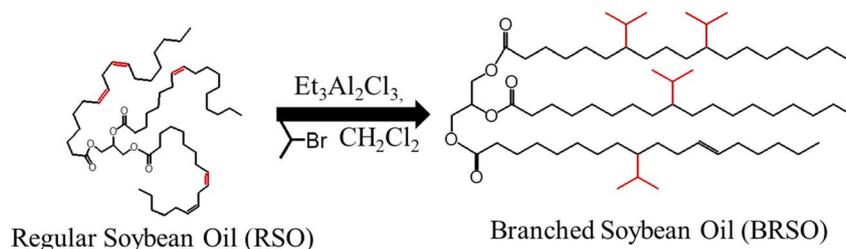
Fig. 1 Synthesis of BRSO via isopropylation of RSO.
