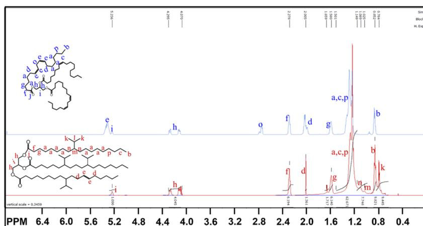
Fig. 3 Comparison between the  $^1\text{H}$  NMR of RSO (top blue line) and BRSO (bottom red line). Spectral peaks are assigned with their corresponding protons in letters.
