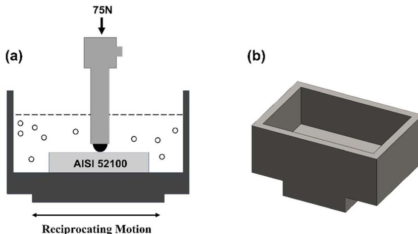
Fig. 2 (a) Schematic representation of the tribological analysis setup. (b) Modified sample holder.
