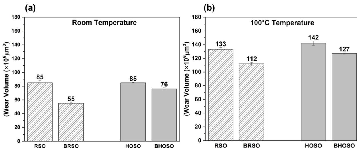
Fig. 7 Comparative wear volume analysis of flat samples (a) room temperature (b) 100 °C temperatures.
