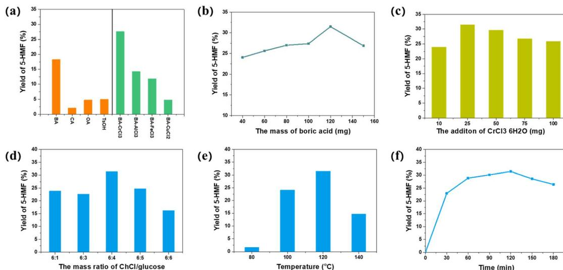
Fig. 3 The change in 5-HMF yield from glucose in ChCl–glucose DES with the reaction condition (a) catalysts types (b) boric acid usages (c)  $\text{CrCl}_3 \cdot 6\text{H}_2\text{O}$  usages (d) ChCl–glucose mass ratios (e) temperature (f) reaction time.
