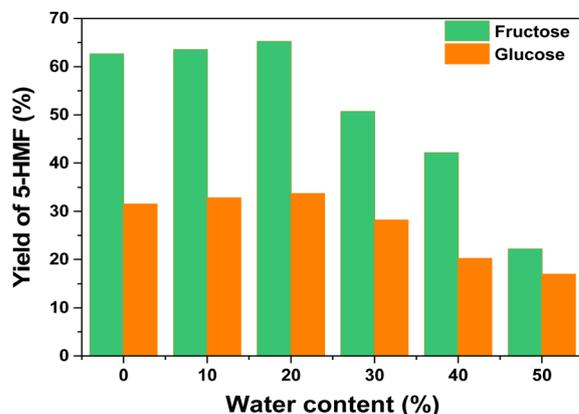
Fig. 5 The effect of water contents on 5-HMF yield in ChCl–fructose and ChCl–glucose DESs under the optimized condition.
