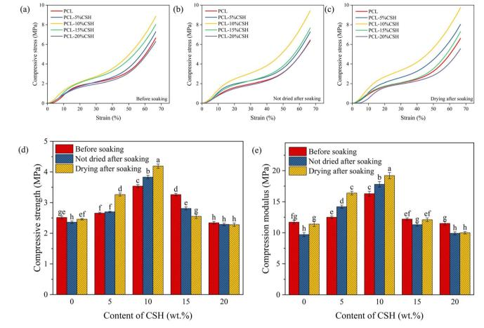
Fig. 4 Compression properties of the different scaffolds at 40% strain. Stress-strain curves of (a) before soaking and (b) not dried after soaking and (c) drying after soaking; (d) strength; (e) modulus.
