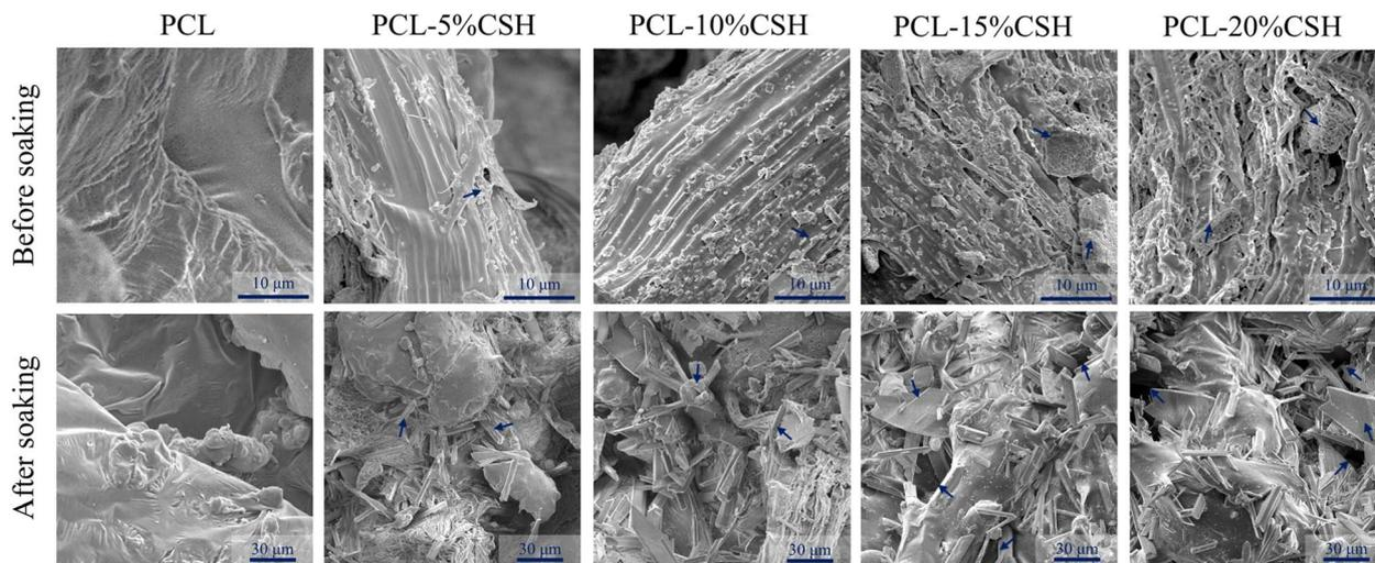
Fig. 6 Tensile fracture morphology of different scaffolds.
