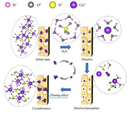
Fig. 7 Self-setting enhancement mechanical mechanism.
