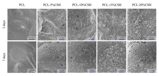
Microscopic morphologies of different scaffolds after soaking in PBS
