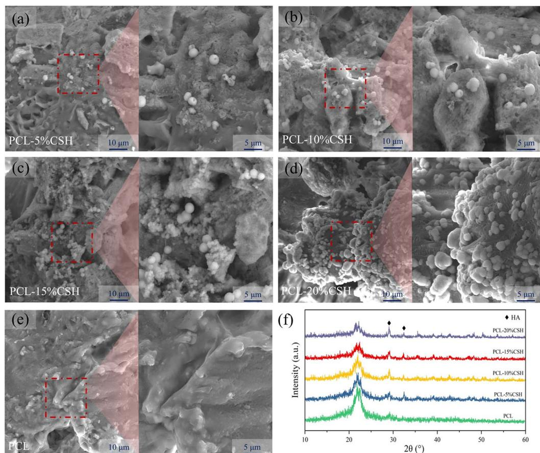
Fig. 11 Surface micromorphology and XRD patterns of the scaffolds after soaking in SBF for 7 days. (a) PCL-5% CSH, (b) PCL-10% CSH, (c) PCL-15% CSH, (d) PCL-20% CSH, and (e) PCL represent the microscopic morphologies of the scaffolds. (f) XRD patterns of the scaffolds.
