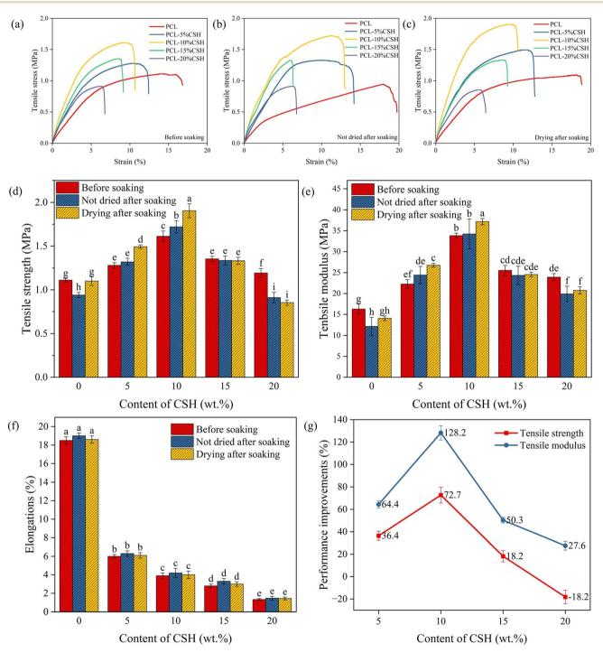
Fig. 3 Tensile properties of different scaffolds. Stress-strain curves of (a) before soaking and (b) not dried after soaking and (c) drying after soaking; (d) strength; (e) modulus; (f) elongation; (g) performance improvement.
