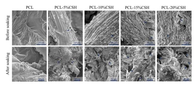
Fig. 6 Tensile fracture morphology of different scaffolds.
