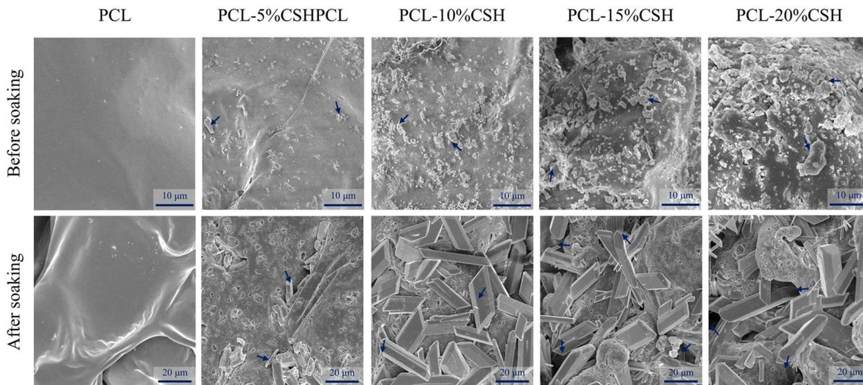
Fig. 5 Microscopic surface morphology of different scaffolds.
