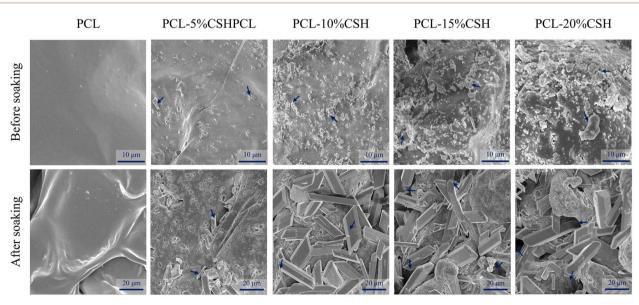
Fig. 5 Microscopic surface morphology of different scaffolds.
