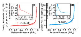
Fig. 8  $N_2$  adsorption—desorption isotherms and pore size distribution of (a) EA-BiOBr and (b) Ch-BiOBr.
