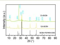
Fig. 4 XRD patterns of EA-BiOBr and Ch-BiOBr.
