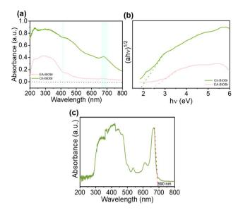
Fig. 6 (a) UV-vis DRS and (b)  $(\alpha h \nu)^{1/2}$  versus  $h \nu$  curves of BiOBr, (c) UV-vis DRS of chlorophyll extracts.
