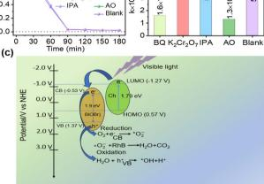
Fig. 10 (a and b) Degradation process and k value of RhB by different scavengers. (c) Mechanism of Ch-BiOBr photocatalytic degradation of RhB.
