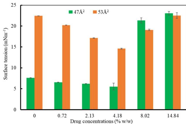
Fig. 5 Impact of drug concentration on the surface tension at constant APL values of 47 Å<sup>2</sup> and 53 Å<sup>2</sup>. A low APL value (47 Å<sup>2</sup>) refers to the molecular area at the exhalation breathing condition and a high APL value (53 Å<sup>2</sup>) indicates the molecular area at the inhalation breathing condition. The estimated errors using block averaging are shown as error bars.
