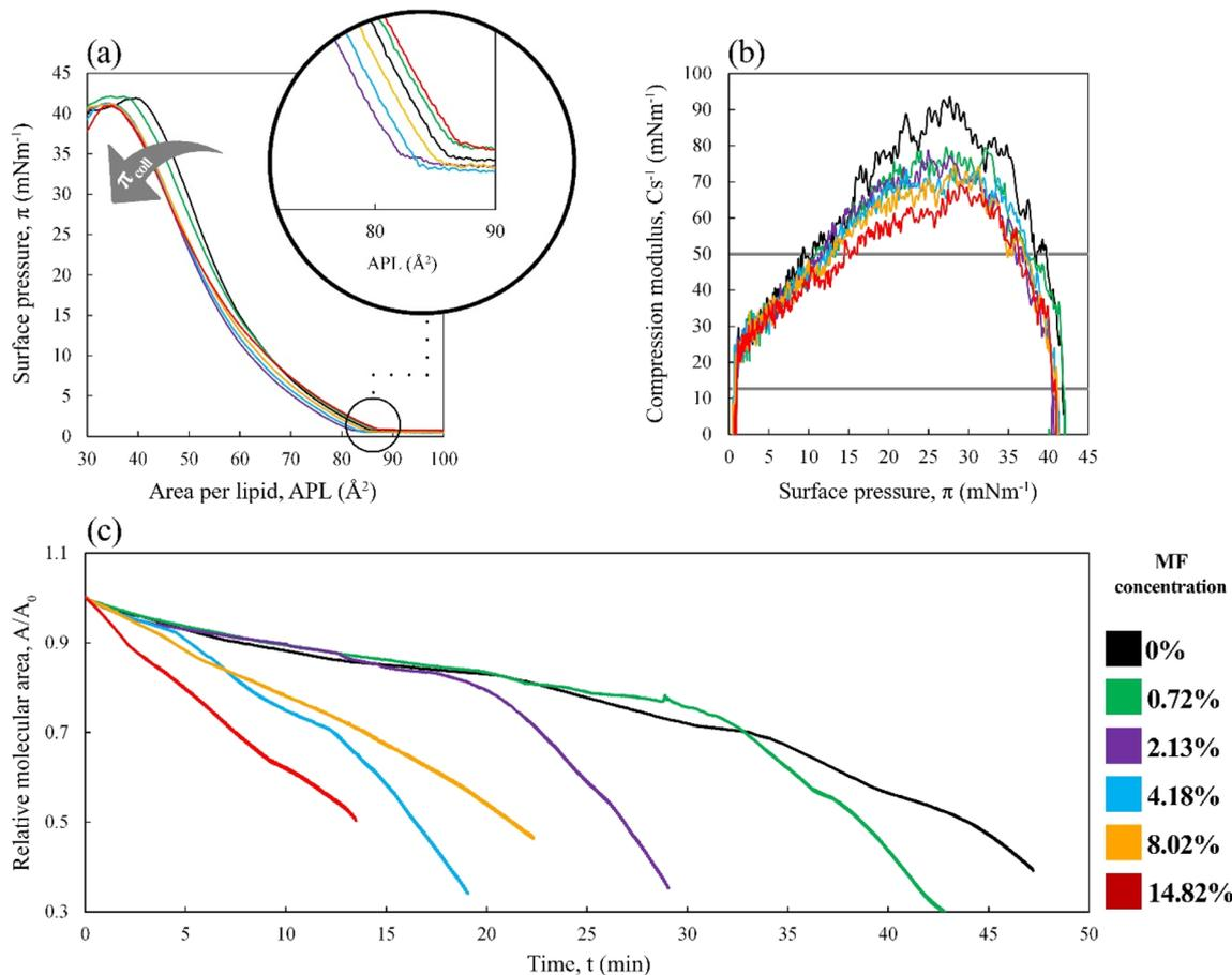
Fig. 1 Effect of various concentrations of mometasone furoate on the mixed Langmuir monolayer of DPPC : POPC : POPG : CHOL, 60 : 20 : 10 : 10 at aqueous subphase at 36.6 °C, (a) the  $\pi$ -APL isotherms (inset): close-up of the initial experimental phase in the  $A_{\text{lift-off}}$  region, (b) the compression modulus vs.  $\pi$ , calculated based on the  $\pi$ -APL isotherms, (c) the relaxation experiments at a constant surface pressure of 30 mN m<sup>-1</sup>.
