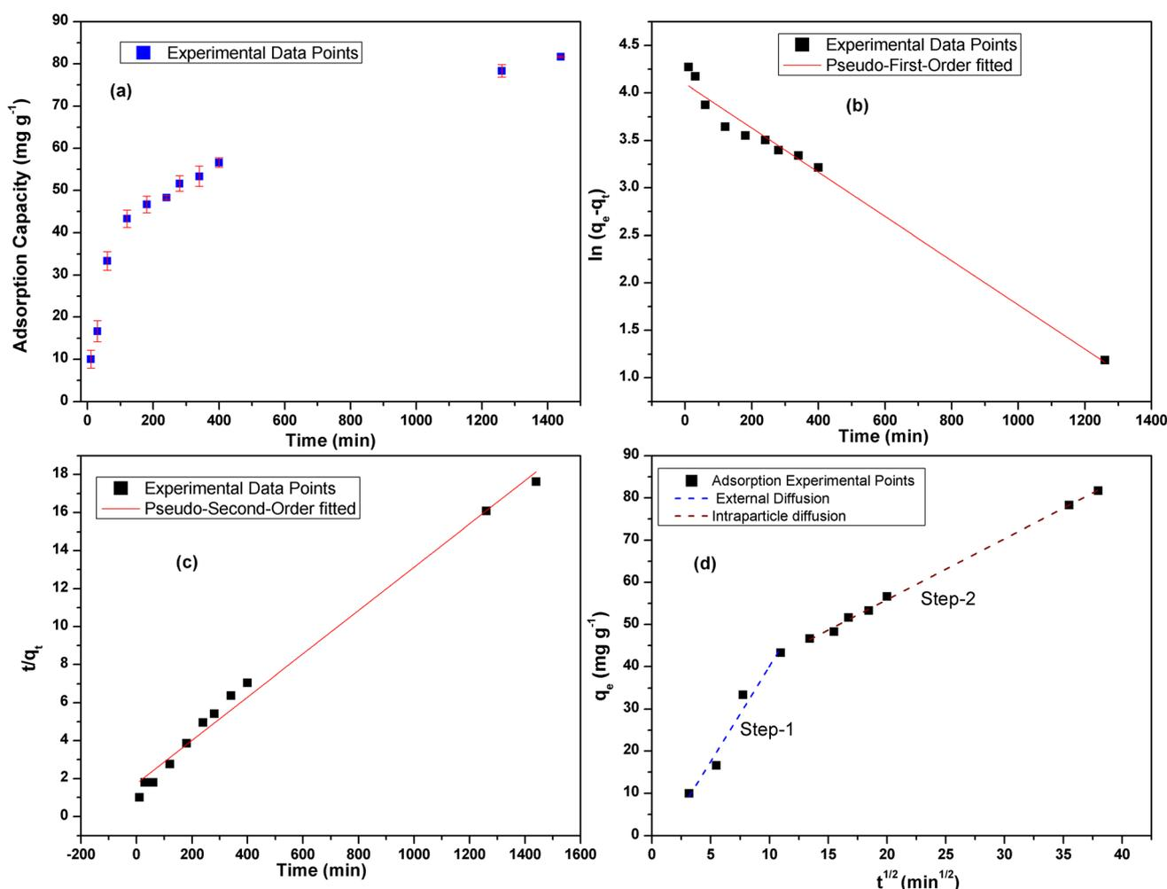
Fig. 3 (a) Variation in  $Cd(II)$  adsorption capacity with change in contact time; experimental points fitted using (b) pseudo-first-order; (c) pseudo-second-order; (d) intraparticle diffusion model. ( $C_0 = 50 \text{ mg L}^{-1}$ ; equilibration time = 10 min–24 h; pH = 6;  $T = 25 \text{ }^\circ\text{C}$ ;  $m/V = 0.3$ ).
