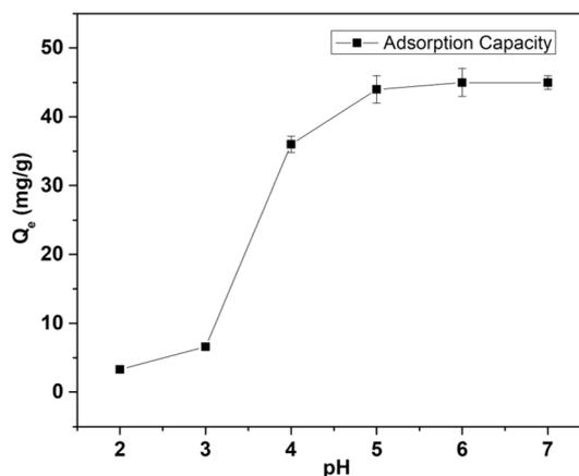
Fig. 2 Variation in  $\text{Cd(II)}$  adsorption capacity of MOF-DSH with change in pH. ( $C_0 = 50\text{ mg L}^{-1}$ ; equilibration time = 5 h; pH = 2–7;  $T = 25\text{ }^\circ\text{C}$ ;  $m/V = 0.3$ ).
