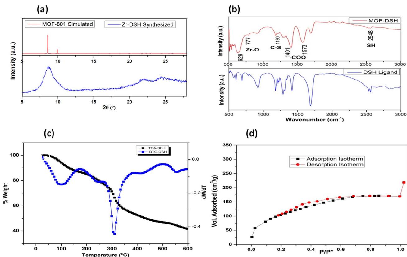
Fig. 1 (a) PXRD pattern of MOF-DSH and simulated pattern of MOF-801 (Zr-succinate); (b) FT-IR spectra of MOF-DSH and DSH (linker); (c) thermogravimetric analysis; (d)  $\text{N}_2$ -adsorption–desorption isotherms.
