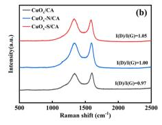
Fig. 7 The XRD patterns and Raman spectra of  $CuO_x/CA$ ,  $CuO_x-N/CA$  and  $CuO_x-S/CA$ . (a): XRD patterns, (b) Raman spectra.
