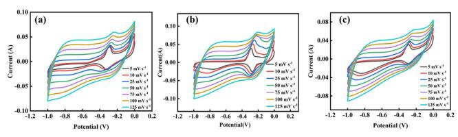
Fig. 1 Cyclic voltammetry curves of copper oxide/carbon composite electrode materials (a) CuO<sub>x</sub>-CA, (b) CuO<sub>x</sub>-N/CA, (c) CuO<sub>x</sub>-S/CA.
