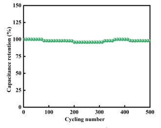
Fig. 3 Cyclic performance diagram of 2 A  $g^{-1}$  of  $CuO_x$ -S/CA.
