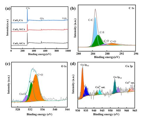
Fig. 9 XPS spectrum of CuO<sub>v</sub>-CA, CuO<sub>v</sub>-N/CA, CuO<sub>v</sub>-S/CA. (a) Full-scan spectrum, (b)-(d) high-resolution spectra of C, O, Cu of CuO<sub>v</sub>-S/CA.
