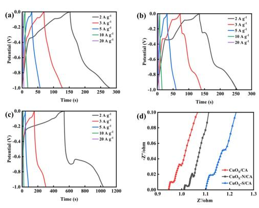
Fig. 2 Galvanostatic charge/discharge curve of copper oxide/carbon composite electrode materials. (a)  $CuO_x/CA$ , (b)  $CuO_x-N/CA$ , (c)  $CuO_x-S/CA$ , (d) AC impedance curve.
