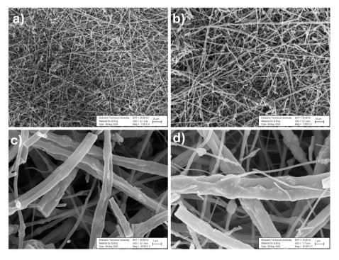
Fig. 2 SEM images of the BTF nanofibers annealed at 500 °C in air for 1 h at different magnifications of 1.0 KX (a), 2.0 KX (b), 20.0 KX and (c and d), in different regions.
