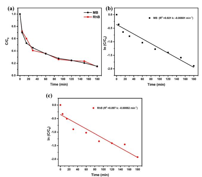
Fig. 4 Photodegradation curves of MB and RhB dyes under simulated sunlight (a) and pseudo-first-order kinetic plots for MB (b) and RhB (c).
