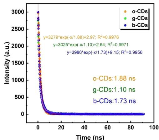
Fig. 6 Fluorescence lifetimes of o-CDs, g-CDs, and b-CDs were tested and calculated at an excitation wavelength of 375 nm.
