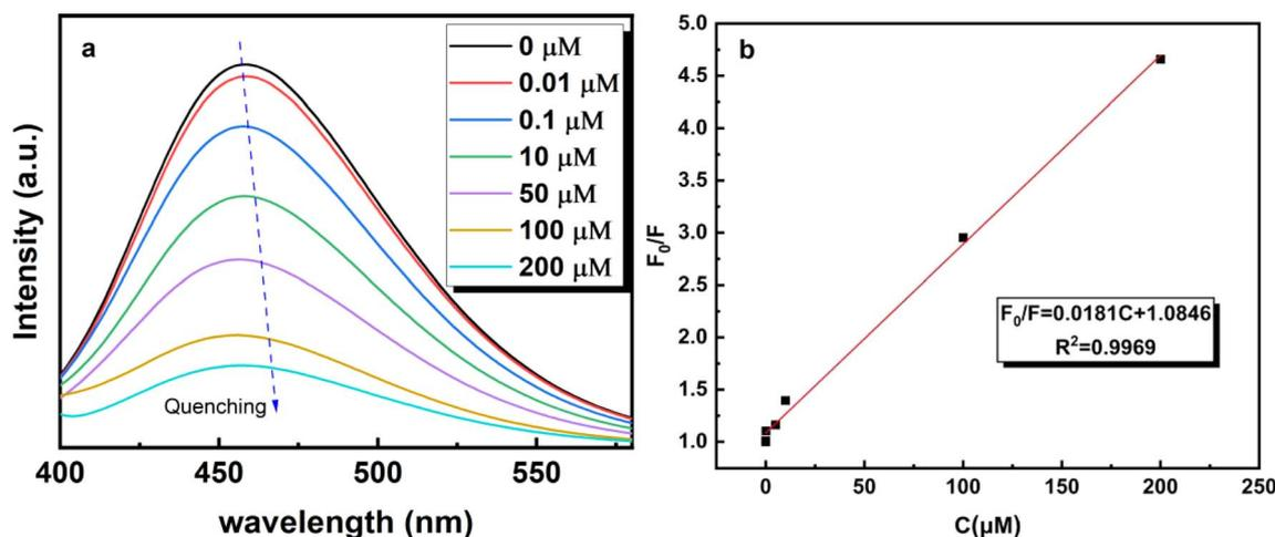
Fig. 9 (a) Fluorescence emission spectra of b-CDs in  $\text{Fe}^{3+}$  solutions with varying concentrations from 0.01 to 200  $\mu\text{M}$ . (b) Fitting curve of  $F_0/F$  as a function of  $\text{Fe}^{3+}$  ion concentration for b-CDs.
