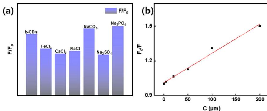
Fig. 10  $F/F_0$  of  $\text{Fe}^{3+}$  detected at  $100 \mu\text{M L}^{-1}$  in 200-fold disturbed water (a); variation of  $\text{Fe}^{3+}$  in the concentration gradient detected in natural water (b).
