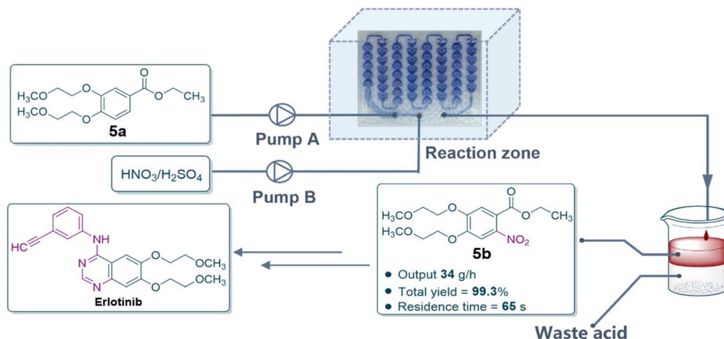
Fig. 4 Continuous-flow synthesis of Erlotinib key intermediate 5b.
