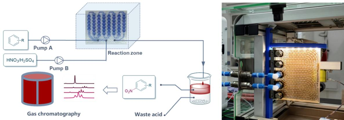
Fig. 2 Continuous-flow reactor setup for condition optimization.
