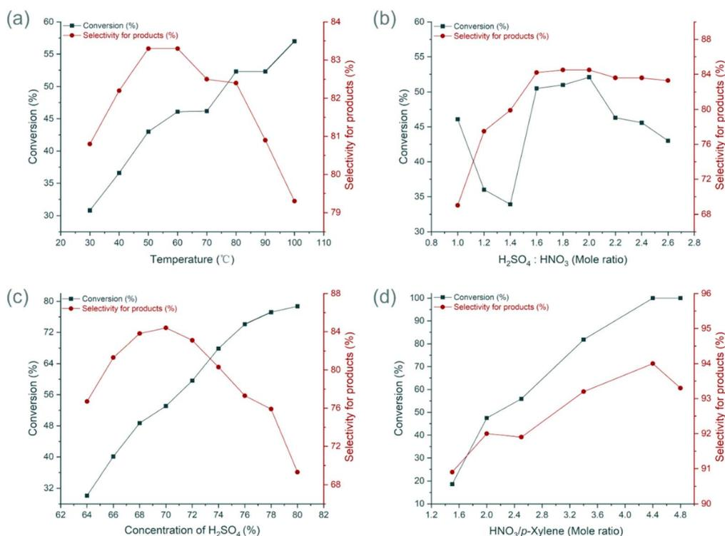
Fig. 3 Optimization of nitration in continuous-flow. (a) The influence of temperature. (b) The influence of mole ratio of  $\text{H}_2\text{SO}_4$  and  $\text{HNO}_3$ . (c) The influence of  $\text{H}_2\text{SO}_4$  concentration. (d) The influence of mole ratio of  $\text{HNO}_3$  and *p*-xylene.
