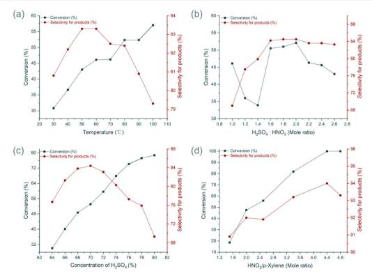
Fig. 3 Optimization of nitration in continuous-flow. (a) The influence of temperature. (b) The influence of mole ratio of  $H_2SO_4$  and  $HNO_3$ . (c) The influence of  $H_2SO_4$  concentration. (d) The influence of  $HNO_3$  and P-xylene.
