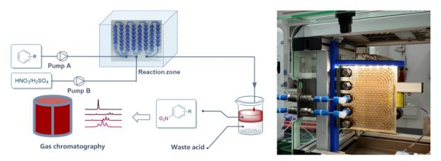
Fig. 2 Continuous-flow reactor setup for condition optimization.
