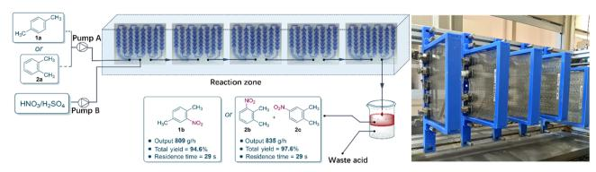
Fig. 5 Continuous-flow scale-up experimental setup.
