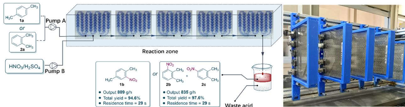
Fig. 5 Continuous-flow scale-up experimental setup.
