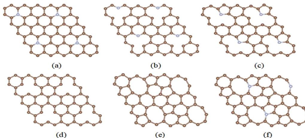
Fig. 1 Structure models of (a) N\_graphitic, (b) N\_pyridinic, (c) N\_pyrrolic, (d) Vac\_C, (e) Vac<sub>2</sub>C, and (f) N\_Vac<sub>2</sub>C. Dark brown and blue represent C and N, respectively.
