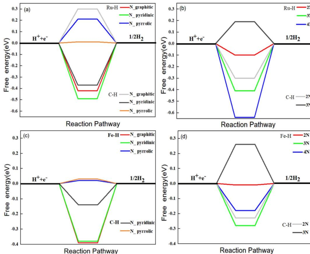
Fig. 5 Calculated HER profile for Ru and Fe SACs on the three different configurations of N-doped graphene substrates (a) Ru@N and (c) Fe@N, and on the 2N to 4N moieties substrates (b) Ru@N<sub>x</sub> and (d) Fe@N<sub>x</sub>.
