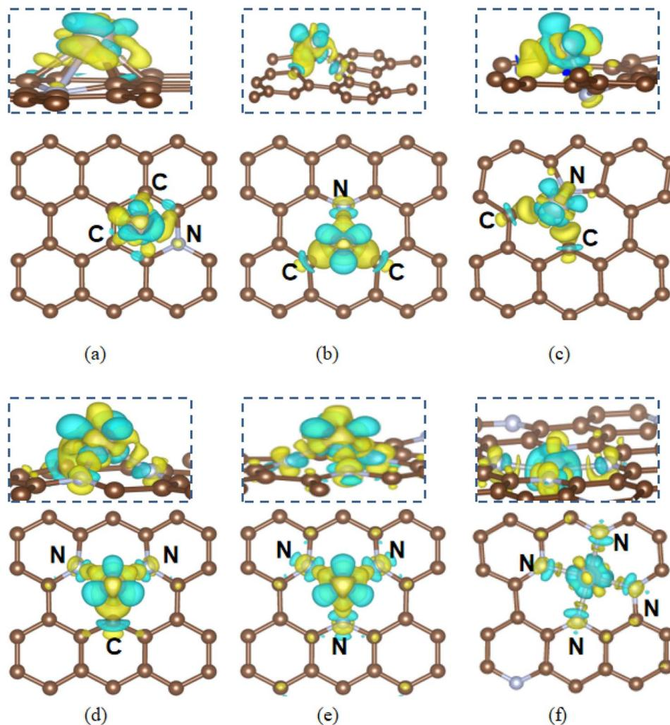
Fig. 3 Electron charge density difference for Ru deposition on the substrates of (a) N\_graphitic, (b) N\_pyridinic, (c) N\_pyrrolic, (d) 2N\_Vac, (e) 3N\_Vac and (f) 4N\_Vac<sub>2</sub> graphene. The yellow and blue areas denote electron accumulation and depletion.
