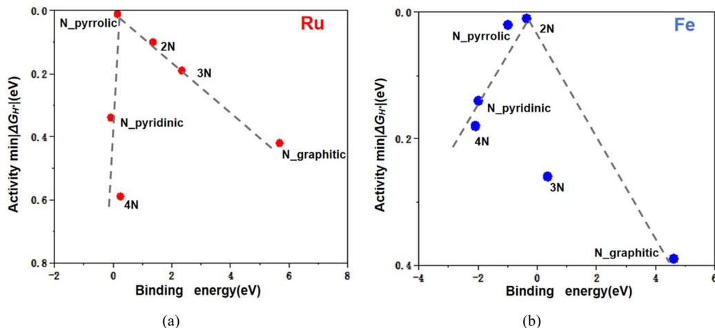
Fig. 7 Volcano plots of catalytic activities as a function of the metal SAC's binding energy on the N-doped graphene substrates: (a) Ru SACs and (b) Fe SACs.
