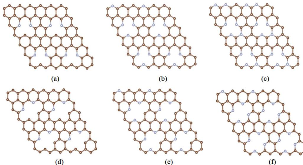
Fig. 2 Structure models of (a) 2N\_Vac, (b) 3N\_Vac, (c) 4N\_Vac, (d) 2N\_Vac<sub>2</sub>, (e) 3N\_Vac<sub>2</sub> and (f) 4N\_Vac<sub>2</sub>. Dark brown and blue represent C and N, respectively.
