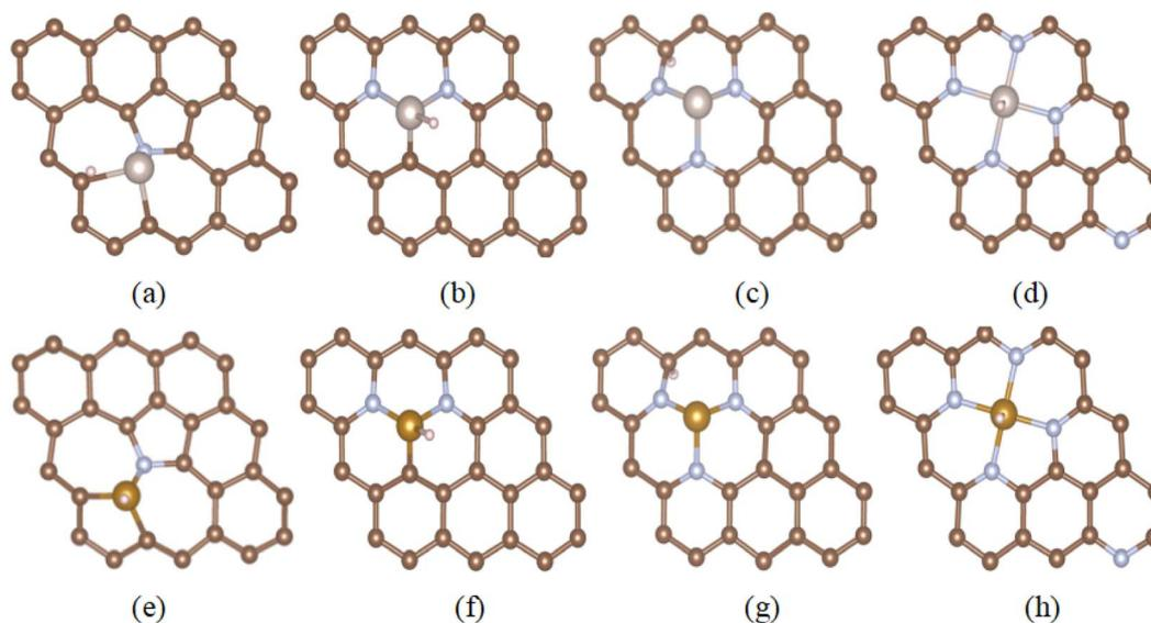
Fig. 6 The optimized hydrogen adsorption configurations at the most active sites on the (a) Ru SAC@N<sub>pyrrolic</sub>, (b) Ru SAC@2N, (c) Ru SAC@3N, (d) Ru SAC@4N, (e) Fe SAC@N<sub>pyrrolic</sub>, (f) Fe SAC@2N, (g) Fe SAC@3N and (h) Fe SAC@4N doped graphene. Dark brown, blue, gray, yellow and white represent C, N, Ru, Fe and H, respectively (side views are given in Fig. S7†).
