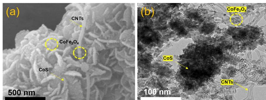
Fig. 3 (a) SEM images and (b) HR-TEM images of CS/CF-CNTs nanocomposite.
