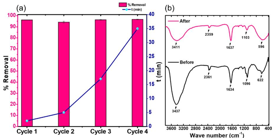
Fig. 11 Reusability of 10 mg/100 mL catalyst for the degradation of 10 mg L<sup>-1</sup> Rhodamine-B at a PMS concentration of 60 mg/100 mL and pH 3.3 (a). FT-IR spectra before and after degradation (b).
