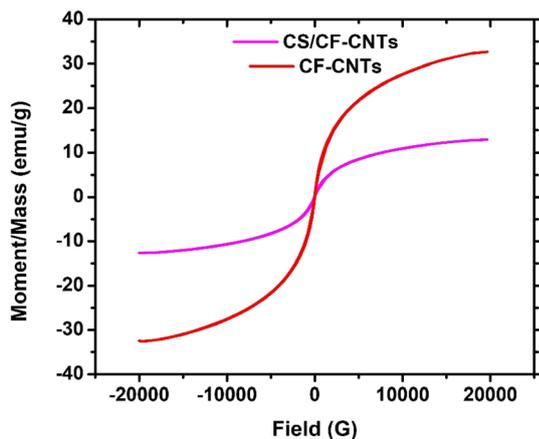
Fig. 5 VSM plots for CS/CF-CNTs and CF-CNTs.
