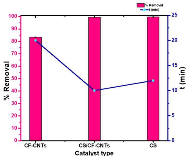
Fig. 7 Comparison between the degradation performance of several catalysts at 10 mg/100 mL catalyst dose and 60 mg/100 mL PMS at normal pH conditions for a Rhodamine-B concentration of 50 ppm.
