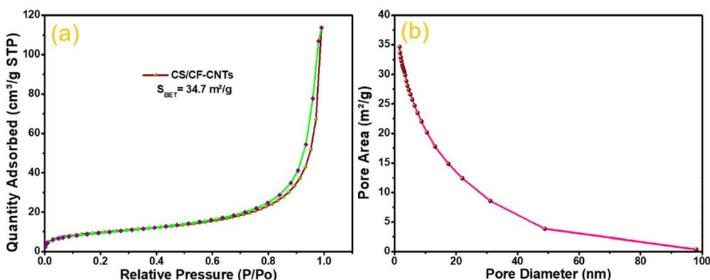
Fig. 6 BET isotherm (a) and pore size distribution (b) of CS/CF-CNTs.
