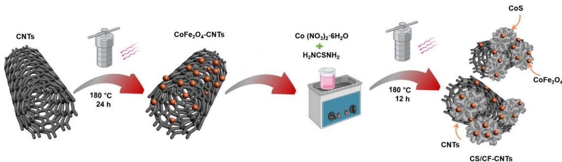
Fig. 1 Schematic diagram of the synthesis of CS/CF-CNTs.
