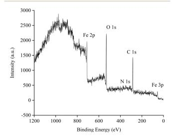
Fig. 11 XPS full spectrum of the carbon steel surface after corrosive treatment using 1 M hydrochloric acid solution containing 40 ppm of corrosion inhibitor.
