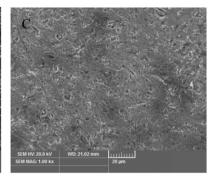
Fig. 10 Scanning electron microscope of carbon steel. (A) The surface of the original uncorroded carbon steel; (B) the surface of carbon steel corroded in 1 M HCl solution without corrosion inhibitor; (C) the surface morphology of carbon steel corroded in 1 M HCl solution with 40 ppm corrosion inhibitor.
