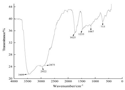
Fig. 1 FTIR of intermediate of IOID.
