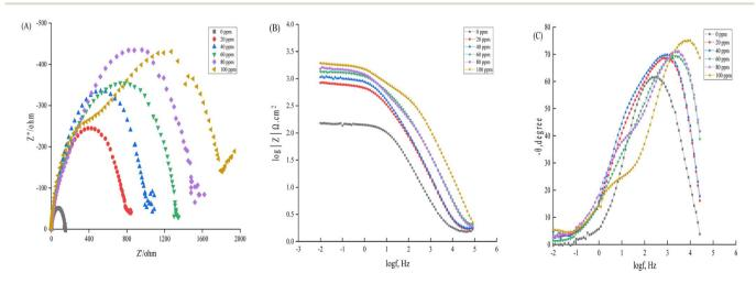
Fig. 7 Nyquist plots (A) and Bode plots (B and C) of carbon steel in hydrochloric acid solution containing different concentrations of IOID (the impedance was normalized by the area).
