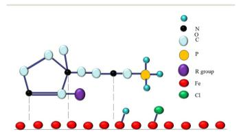
Fig. 13 Schematic illustration of the adsorption mechanism of corrosion inhibitor on the carbon steel surface.
