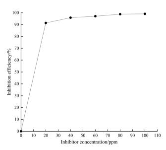
Fig. 3 Effect of IOID concentration on the inhibition of carbon steel in HCl solution.
