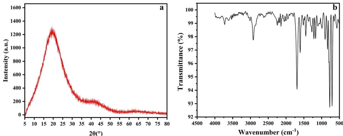
Fig. 5 Characterization of our synthesized DVB particles by (a) XRD and (b) FTIR.
