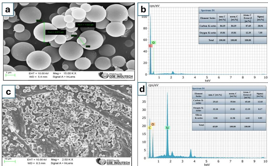
Fig. 4 The morphological characterization of synthesized polymer DVB particles using FE-SEM (a) synthesized DVB polymer particle size ranged from 1–5  $\mu\text{m}$ , (b) the EDX analysis of the synthesised polymer DVB (c) morphology of DVB/PDMS/CNT coated patches, and (d) the EDX analysis of the DVB/PDMS/CNT coated patches.
