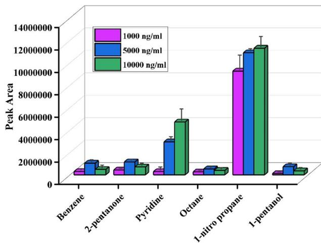
Fig. 7 Headspace validation of p-TF-SPME by McReynolds standard solution.
