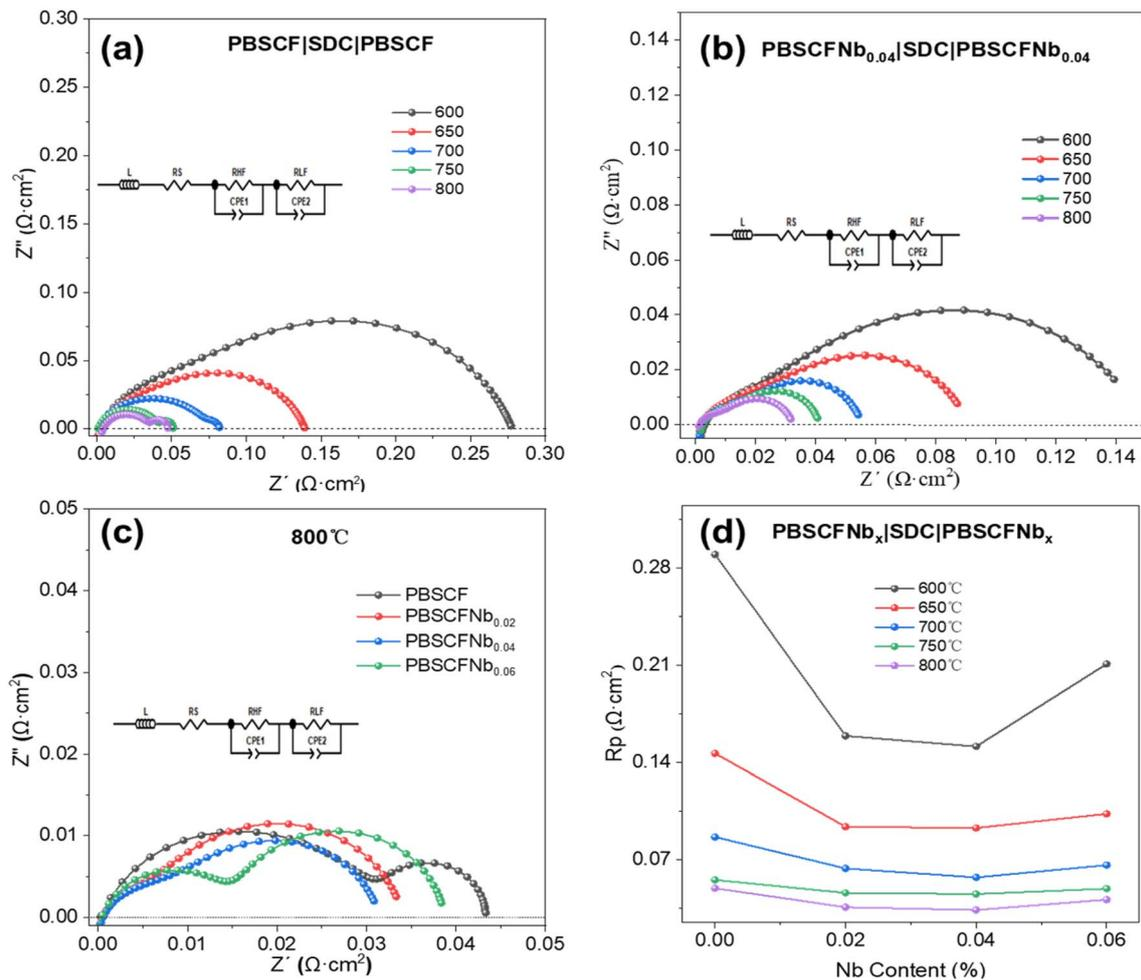
Fig. 7 ASR shows the temperature dependence of (a) PBSCF, (b) PBSCFNb<sub>0.04</sub>, (d) PBSCFNb<sub>x</sub>, and an (c) ASR diagram of PBSCFNb<sub>x</sub> at 800 °C.
