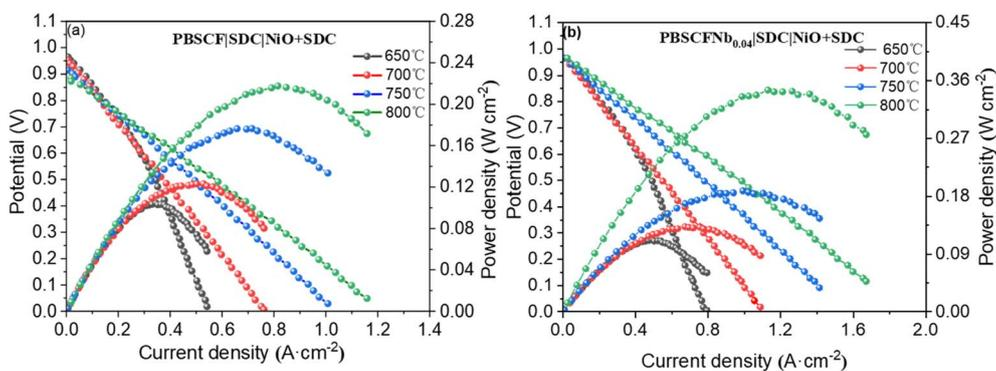
Fig. 8 (a) The power density of a single cell PBSCF|SDC|Ni + SDC at 650–800 °C and (b) the power density of single cell PBSCF<sub>0.04</sub>|SDC|Ni + SDC at 650–800 °C.
