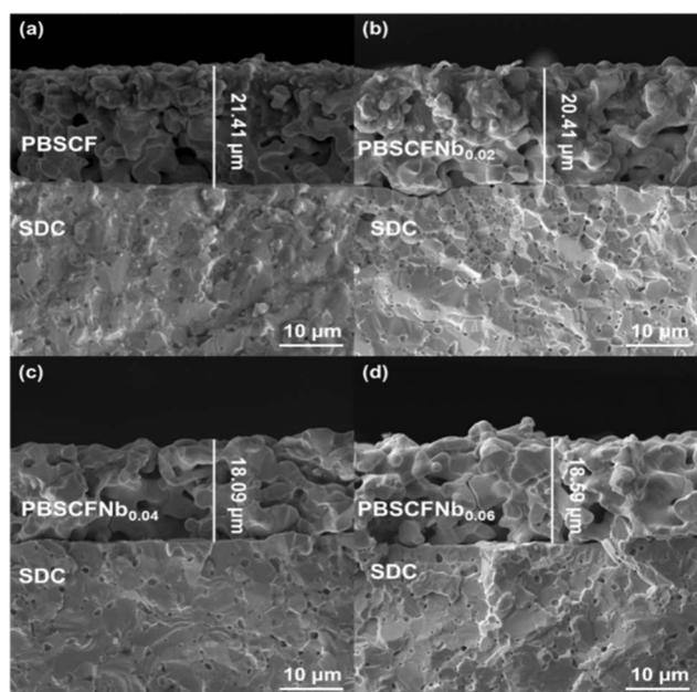
Fig. 5 Cross-section of SEM images of (a) PBSCF, (b) PBSCFNb<sub>0.02</sub>, (c) PBSCFNb<sub>0.04</sub>, and (d) PBSCFNb<sub>0.06</sub>.
