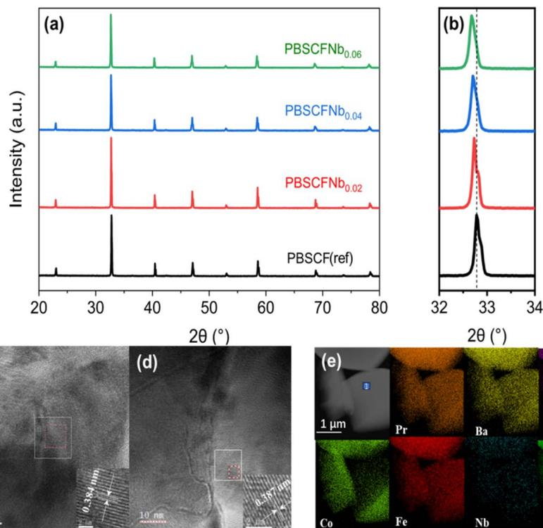
Fig. 1 (a) XRD patterns of PBSCFNb<sub>x</sub> cathode materials. (b) Magnified XRD patterns of PBSCFNb<sub>x</sub>. (c) High-resolution TEM of PBSCF. (d) High-resolution TEM of PBSCFNb<sub>0.04</sub>, and (e) EDS of PBSCFNb<sub>0.04</sub>.
