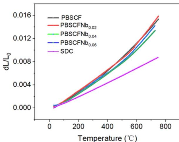
Fig. 2 The thermal expansion of PBSCFNb<sub>x</sub> and SDC.
