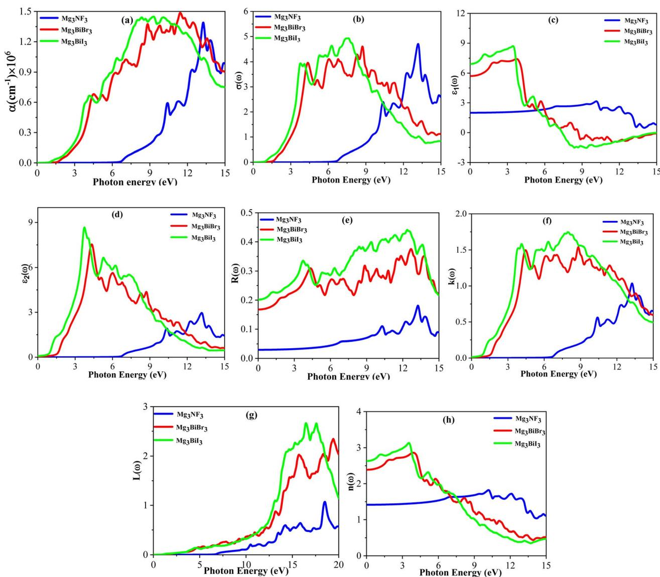
**Fig. 6** Calculated optical parameters (a) absorption coefficient, (b) conductivity, (c) real dielectric part, (d) imaginary dielectric part, (e) reflectivity, (f) extinction coefficient, (g) loss function and (h) refractive index of  $\text{Mg}_3\text{AB}_3$  (A = N, Bi; B = F, Br, I).
