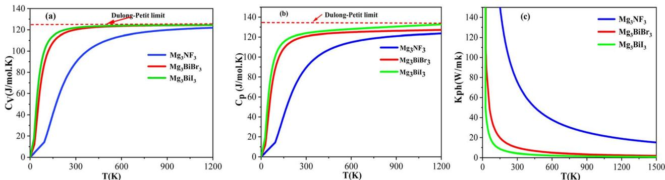
**Fig. 7** The temperature-dependent specific heats (a)  $C_v$  at constant volume (b)  $C_p$  at constant pressure and (c) lattice thermal conductivity of  $\text{Mg}_3\text{AB}_3$  (A = N, Bi; B = F, Br, I) perovskite compounds.
