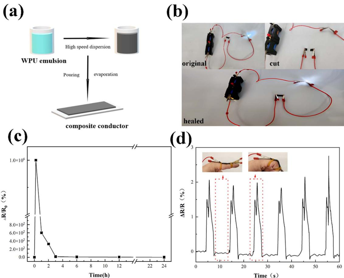
Fig. 6 (a) Preparation of composite conductors. (b) Schematic diagram of the healing of the  $D_8A_2$ WPU-CNT composite conductor with LEDs in series. (c)  $\Delta R/R_0$  for different times of healing at 100 °C. (d)  $D_8A_2$ WPU-CNT flexible strain sensor detects  $\Delta R/R_0$  vs. finger movement time.
