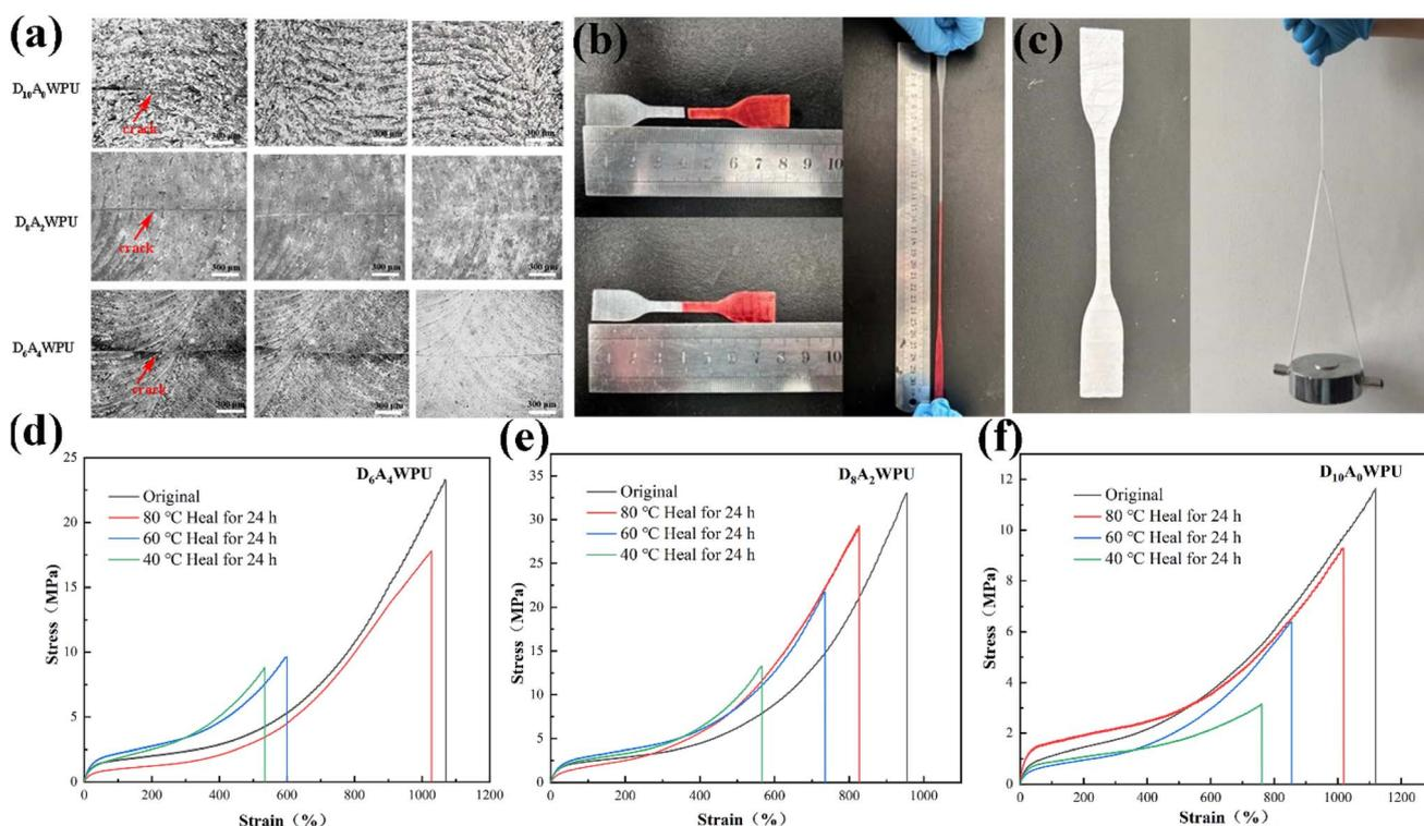
Fig. 4 (a) Scratch healing of  $D_{10}A_0$ WPU,  $D_8A_2$ WPU and  $D_6A_4$ WPU at 80 °C for different time.  $D_8A_2$ WPU after 6 h healing at 80 °C (b) tensile test and (c) loaded with 2.5 kg weights. Stress–strain curves of (d)  $D_6A_4$ WPU, (e)  $D_8A_2$ WPU, (f)  $D_{10}A_0$ WPU healed for 24 hours at 40 °C, 60 °C, 80 °C.
