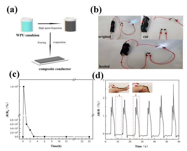
Fig. 6 (a) Preparation of composite conductors. (b) Schematic diagram of the healing of the D<sub>8</sub>A<sub>2</sub>WPU-CNT composite conductor with LEDs in series. (c)  $\Delta R/R_0$  for different times of healing at 100 °C. (d) D<sub>8</sub>A<sub>2</sub>WPU-CNT flexible strain sensor detects  $\Delta R/R_0$  vs. finger movement time.
