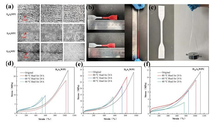
(a) Scratch healing of  $D_{10}A_0WPU$ ,  $D_8A_2WPU$  and  $D_6A_4WPU$  at 80 °C for different time.  $D_8A_2WPU$  after 6 h healing at 80 °C (b) tensile test and (c) loaded with 2.5 kg weights. Stress-strain curves of (d)  $D_6A_4WPU$ , (e)  $D_8A_2WPU$ , (f)  $D_{10}A_0WPU$  healed for 24 hours at 40 °C, 60 °C, 80 °C.
