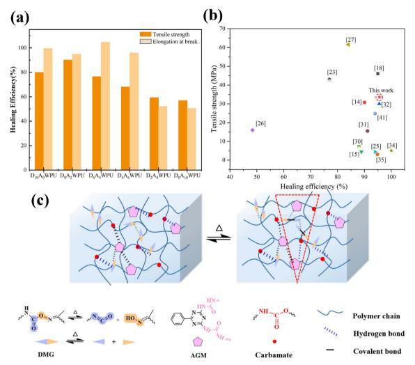
Fig. 5 (a) Self-repair efficiency of  $D_xA_yWPU$  repaired at 80 °C for 24 h. (b) Comparison of tensile strength and healing efficiency for the representative  $D_8A_2WPU$  films in this work and other self-healable polymers reported in literature. (c) Schematic diagram of the self-healing mechanism of  $D_xA_yWPU$  films.
