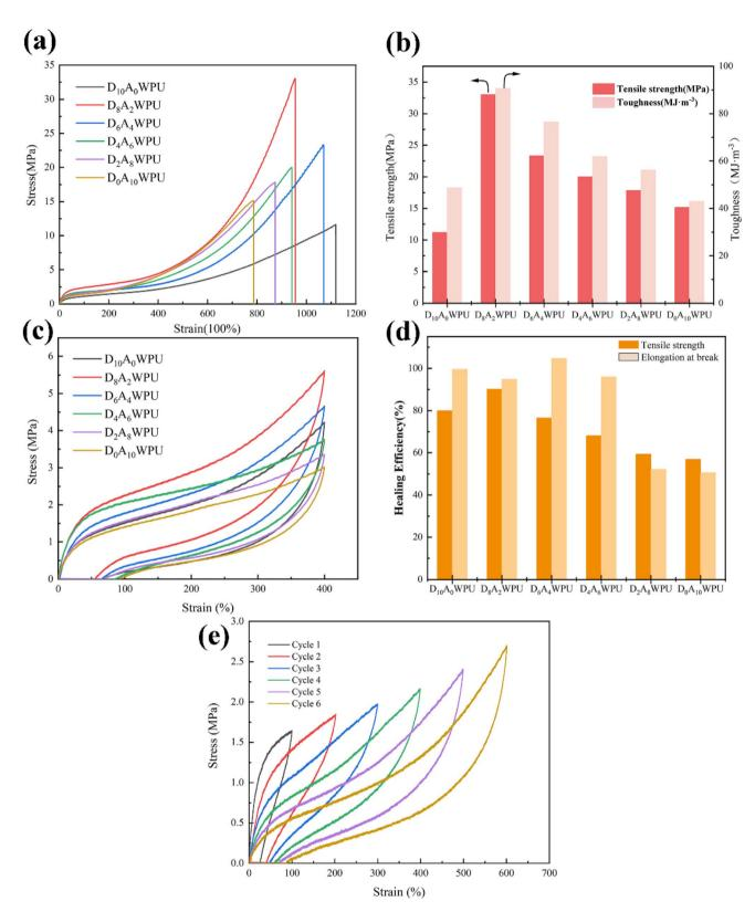
Fig. 3 (a) Stress-strain curves of  $D_xA_yWPU$ . (b) Tensile strength and toughness of  $D_xA_yWPU$ . (c) Hysteresis curves of  $D_xA_yWPU$  specimen at 400% fixed strain with different loading-unloading times. (d) Residual strain and hysteresis energy of  $D_xA_yWPU$ . (e) Cyclic tensile curve of  $D_8A_2WPU$  at 100–600% strain.
