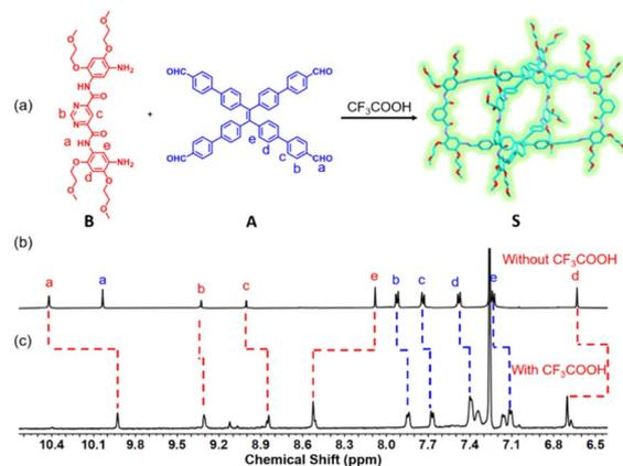
Fig. 1 (a) Synthesis of the supramolecular cage **S**, and the comparison of the <sup>1</sup>H NMR spectra of (b) a mixture of ligands **A** and **B** and (c) cage **S**.
