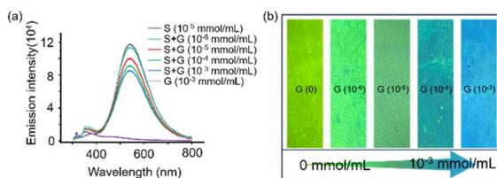
Fig. 2 (a) Fluorescence spectra of **G** with different concentrations added to **S** ( $10^{-5}$  mol L $^{-1}$ ). (b) Images of test papers dipped with **S** ( $10^{-5}$  mmol mL $^{-1}$ ) in different concentrations of **G** under 365 nm UV light.
