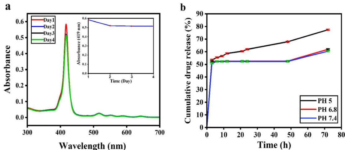
Fig. 5 (a) Spectroscopic evaluation of the synthesized CDs' water stability. (Inset) Plotting of the maximum absorbance value (at  $\lambda = 419$  nm) against the corresponding time. (b) *In vitro* pH-dependent DOX release from the DOX@CDs nanocomposite at pH 5.0, 6.8, and 7.4, data are expressed as SD of mean and  $n = 3$ .
