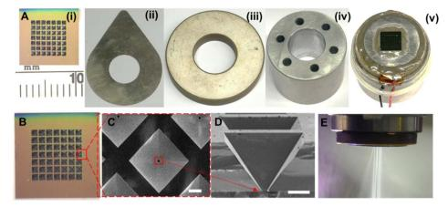
Fig. 1 Assembly of the microparticle production head components; (A) images of microparticle producer head components: (i) microfabricated spray nozzle array, (ii) metal disc, (iii) ultrasonic (piezoelectric) transducer, (iv) solution reservoir, (v) assembled microparticle production head. (B) A magnified image of a microfabricated spray nozzle array. (C and D) SEM image of a single nozzle (scale bars show 200  $\mu$ m). (E) Image of an operating microparticle production system.
