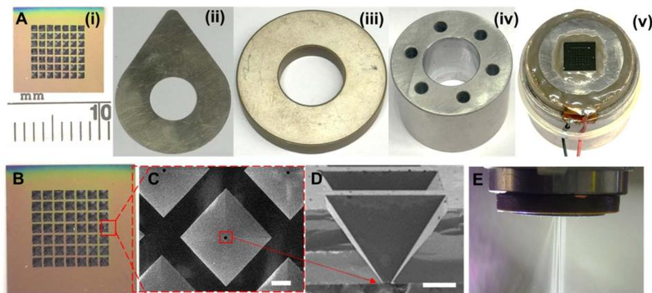
**Fig. 1** Assembly of the microparticle production head components; (A) images of microparticle producer head components: (i) microfabricated spray nozzle array, (ii) metal disc, (iii) ultrasonic (piezoelectric) transducer, (iv) solution reservoir, (v) assembled microparticle production head. (B) A magnified image of a microfabricated spray nozzle array. (C and D) SEM image of a single nozzle (scale bars show 200  $\mu\text{m}$ ). (E) Image of an operating microparticle production system.
