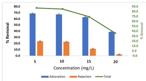
Fig. 14 The influence of feed solution concentration on the removal of Cr(VI).
