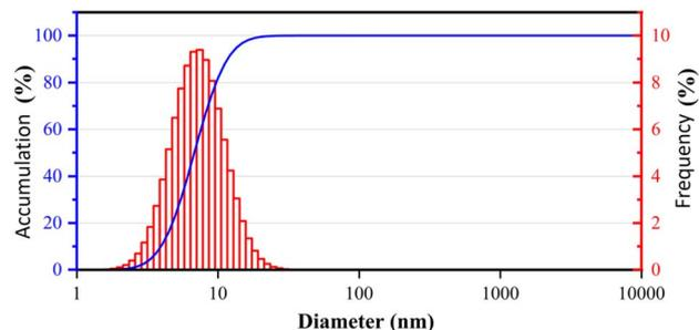
Fig. 4 The particle size distribution results of B-polyphenol.
