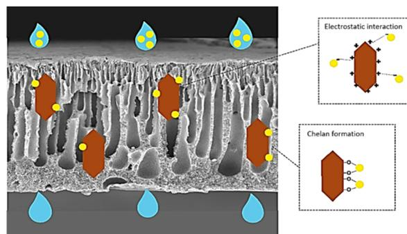
Fig. 17 Illustration of the Cr(vi) removal mechanism.
