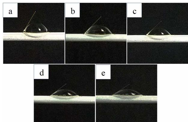
Fig. 10 Contact angle of M0 (a); M0.5 (b); M1 (c); M1.5 (d); and M2 (e).
