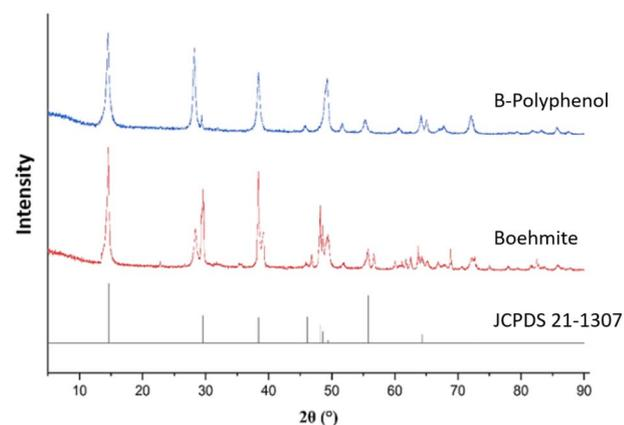
Fig. 3 XRD spectra of boehmite and B-polyphenol.
