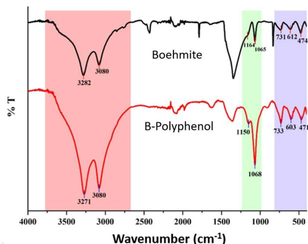
Fig. 5 FTIR spectra of boehmite and B-polyphenol.
